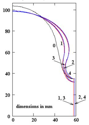
Fig. 1. Original TESLA cell shape (0) and optimized shapes: 1, 3 -  $\Psi$  = 0; 2, 4 -  $\Psi$  = 3.4°; 1, 2 -  $R_a$  = 32 mm;, 3, 4 -  $R_a$  = 35 mm.
