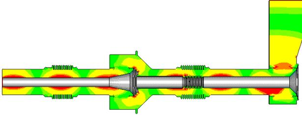
Figure 5: Electric fields in the coupler.
