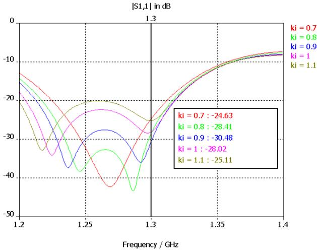
Figure 4: Reflection of the coupler in a frequency range at different coupling (coupling increases from weak to strong when  $k_i$  varies from 0.7 to 1.1).
