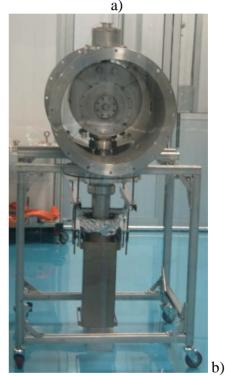
Figure 6: a) 3D view of the input coupler test cryostat with coupling cavity and two couplers; b) the cryostat being assembled in the clean room.
