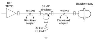
Figure 1: Configuration of the buncher cavity RF system.
