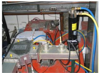
Figure 4: 20 kWCW AFT circulator with RF load.
