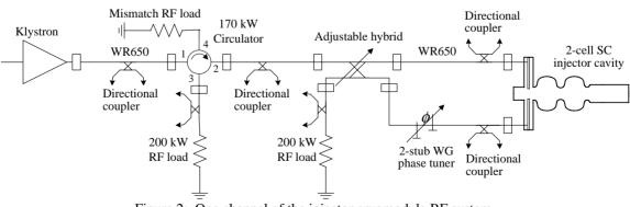
Figure 2: One channel of the injector cryomodule RF system.
