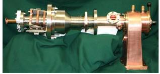
Figure 5: ERL injector cryomodule input coupler.
