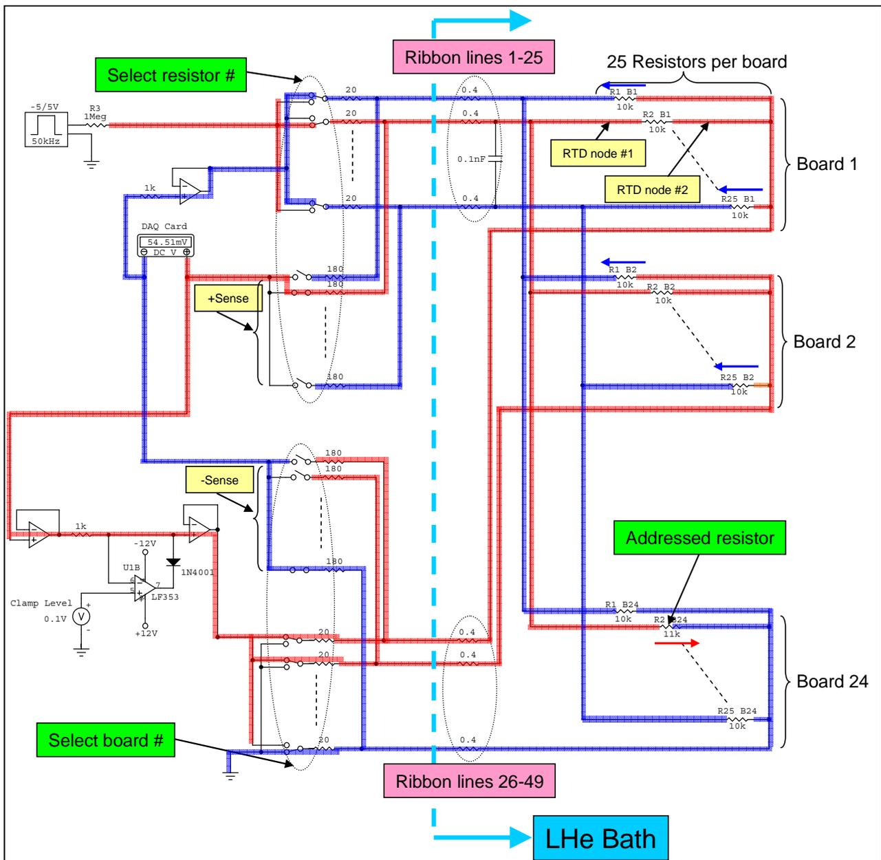
Figure 2: A simplified schematic representing the RTD sensor boards, the ribbon cables, and the signal processing circuit external to the helium dewar.
