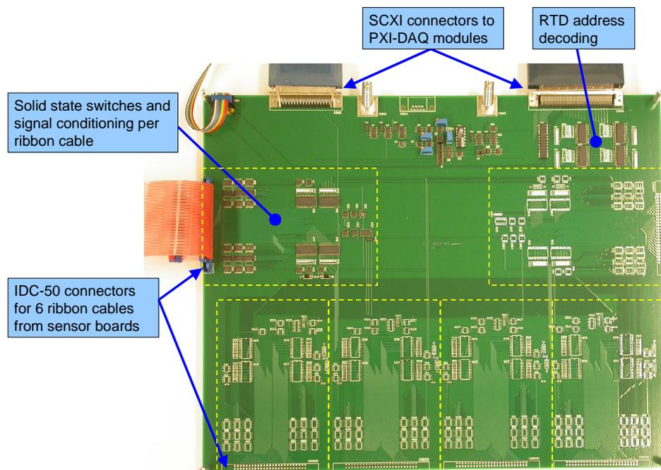
Figure 3: Layout of the switching and signal processing pc board.
