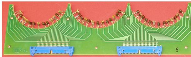
Figure 1: An RTD sensor pc board contoured to match the shape of an SRF cavity.
