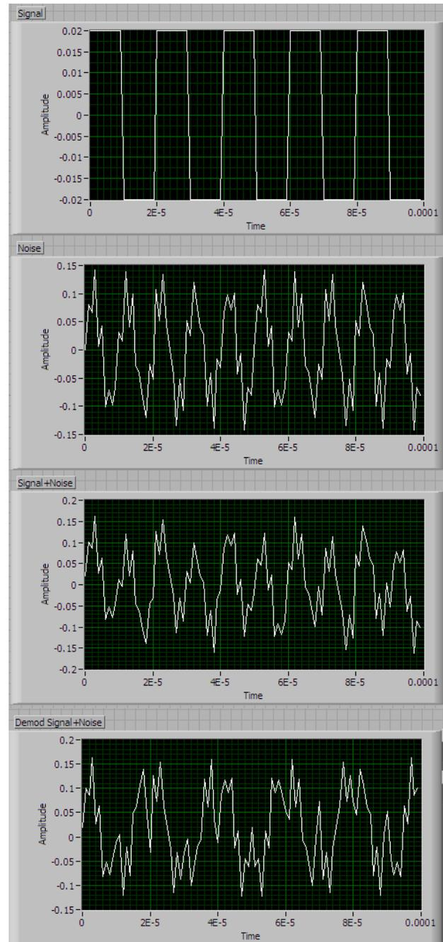
Figure 4: Illustration of the lock-in demodulation technique for parameters considered for this multiplexed RTD data acquisition system. Summing all of the data points in the demodulated fourth trace recovers the 20 mV amplitude of the desired signal in the top trace to <0.1% accuracy.
