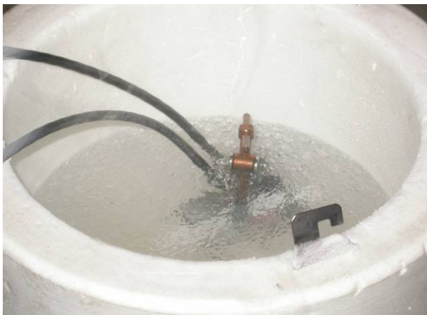
Figure 2: Measurement of DC conductivity at 77K in liquid nitrogen.
