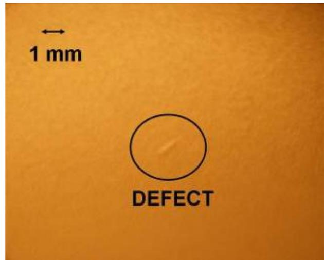
Figure 5: Defect located with second sound.
