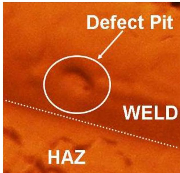
Figure 6: Defect located with second sound on a cavity equator weld. The defect is circled and the weld and heat affected zone (HAZ) are labeled [9].
