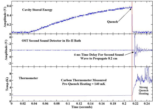
Figure 4: A single quench event measured with an OST in the He-II bath 8.2 cm away from the cavity defect and with a carbon thermometer attached to the cavity surface 2 cm away from the cavity defect.
