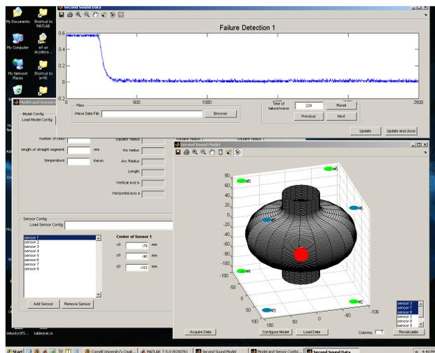
Figure 7: An automated second sound data acquisition and analysis software package is being developed for even easier quench-spot location.
