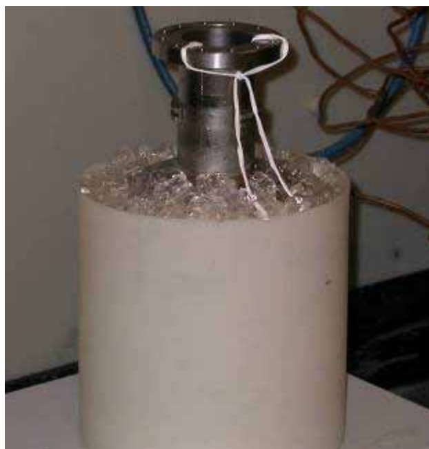
Figure 1: BCP of a single-cell Niowave cavity packed in ice. The white Teflon rope supports a Niobium sample inside the cavity for material removal measurements.
