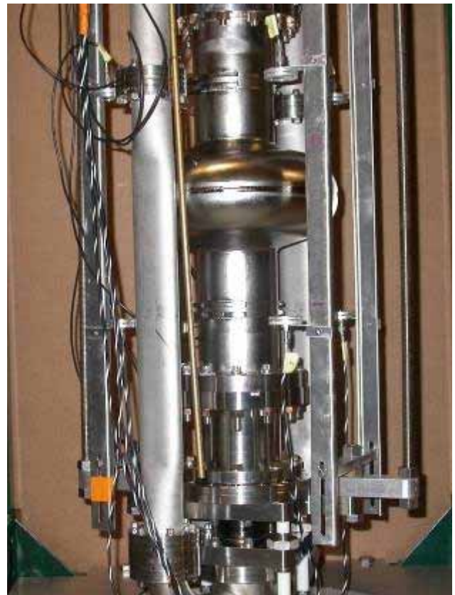
Figure 3: A single-cell cavity ready for testing. Six of the eight oscillating superleak transducers are visible.
