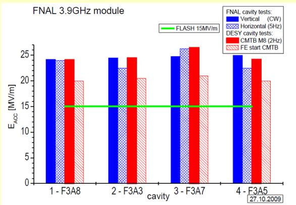
Performance results comparison for vertical test, horizontal test at FNAL, and cryomodule test at DESY.
