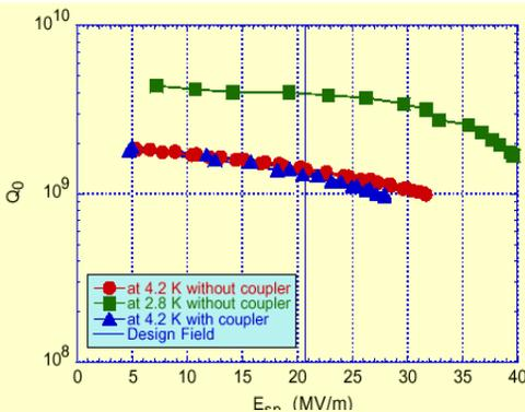
Performance of 500 MHz crab cavity The design kick is 1.44 MV, corresponding to peak surface fields of 21 MV/m and 60 mT.
