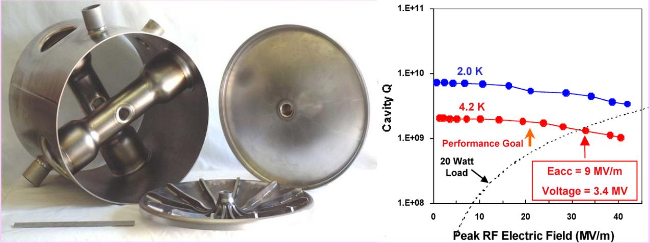
Argonne, 345 MHz ,  $\beta = 0.4$ , double Spoke Resonator.
