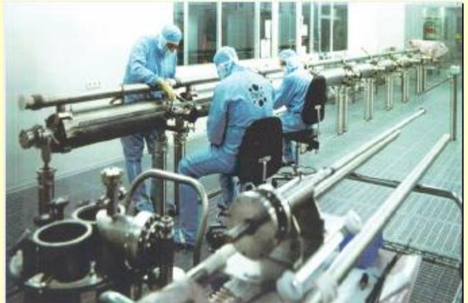
Cavity string assembly in clean room at DESY.
