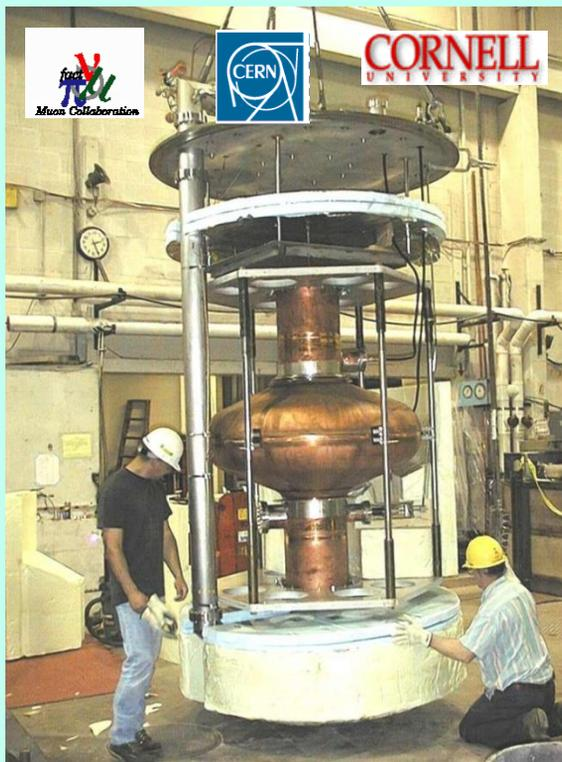
A CERN-Cornell collaboration designed, fabricated and tested a 200 MHz single cell Nb-Cu cavity. In the first such unit, an accelerating field of 10 MV/m was reached at a Q near  $10^9$ . The neutrino factory and the muon collider call for several hundred meters of 200 MHz cavities to provide gradients of 15 MV/m. Nb-Cu is the technology of choice driven by the cost concern. The success of 400 MHz LHC cavities in reaching comparable gradients is encouraging.
