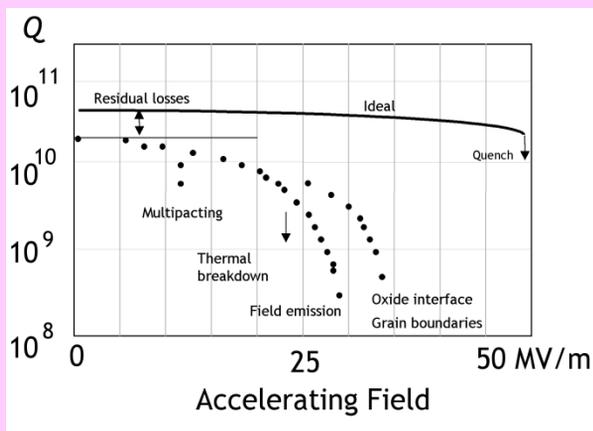
Ideally we would expect the cavity Q to remain constant (at the BCS predicted value) as the field increases, until the quench field. However, as surface electric and magnetic fields rise, several effects set in to drop the Q. These are multipacting, thermal breakdown, medium field slope, field emission, and high field Q-drop. Most of these effects are now understood and solutions invented.
