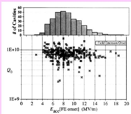
Distribution of gradients and  $Q_0$  at the onset of field emission for more than 300 CEBAF cavities tested in the early 1990's. The average gradient is 8.7 MV/m.
