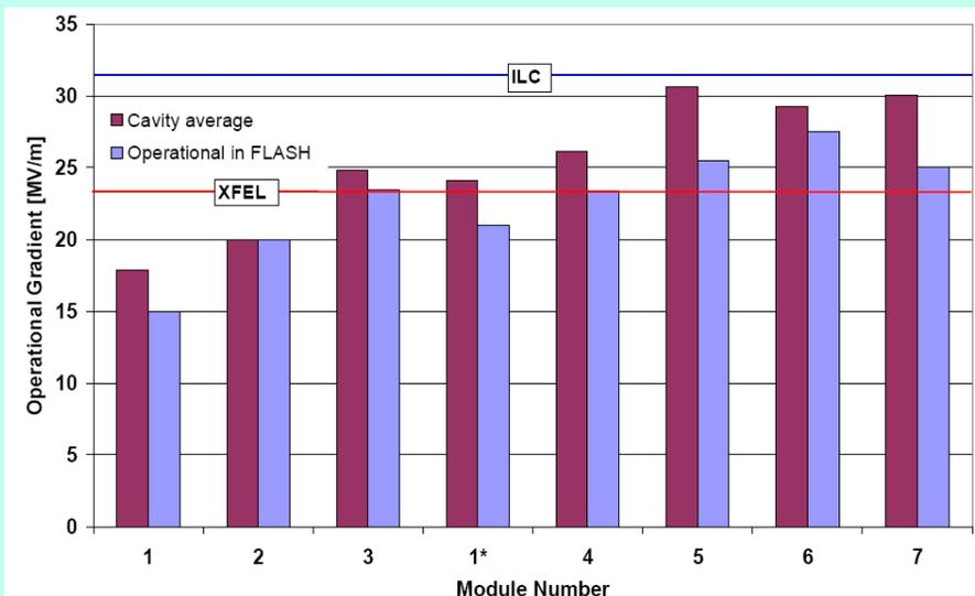
Steady advance in cryomodule gradients at DESY.
