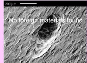
Typical examples of quench-producing defects located by temperature mapping and imaged by SEM are: chemical stains, foreign metal inclusions, pits with sharp edges, metal burrs from scratches, voids or delaminated regions of Nb, weld beads and other types of welding mistakes. 0.1 to 1 mm size defects cause thermal breakdown.
