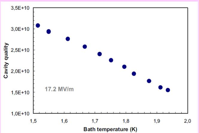
High Q values for a 9-cell cavity measured in the BESSY test cryomodule.
