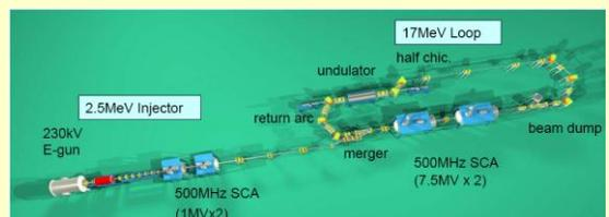
The JAEA FEL runs with 500 MHz superconducting cavities .
