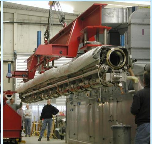
Cryomodule assembly at DESY.
