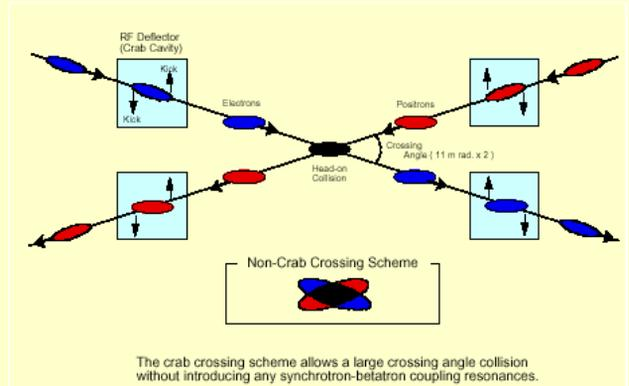
The crab crossing scheme tilts the bunches to provide head-on collisions.
