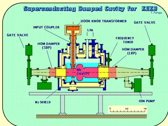
KEK-B cavity and cryomodule.
