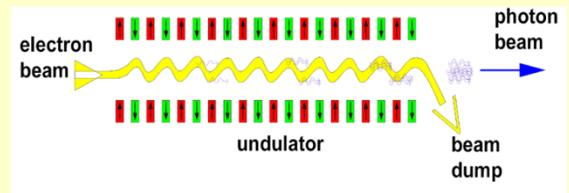
The SASE principle : A short bunch of high intensity interacts with the undulator field of a long wiggler.
