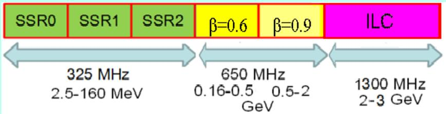
Schematic layout for the Fermilab Project X (formerly Proton Driver) SSR is single spoke resonator. ILC section has nearly ILC compatible cavities.
