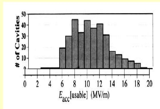
Usable gradients for CEBAF cavities at first installation. Most of the 42 cryomodules have been kept permanently cold since 1995. From October 2000 through June of 2001, CEBAF delivered more than 4500 beam hours for physics. SRF cavity related faults accounted for less than 0.5% down time. Cavity gradients are being steadily upgraded by re-processing from 7 to 15 MV/m.
