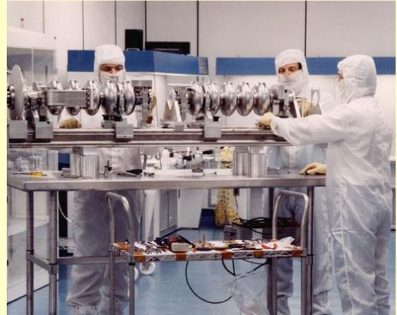
CEBAF 5-cell cavities operate at 1497 MHz with an active length of 50 cm each. There are eight cavities per cryomodule. The cavity design chosen for CEBAF was based on a Cornell design developed for storage rings. It met gradient and  $Q_0$  requirements, damped higher-order modes well, and was proven in a beam test at CESR.
