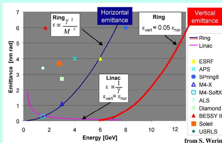
A comparison of vertical and horizontal emittances for rings and linacs.
