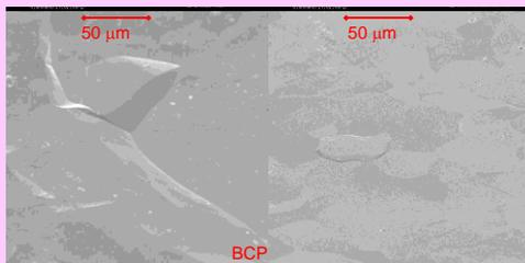
Comparison of a niobium surface prepared by (left) standard chemical polishing and (right) electropolishing.
