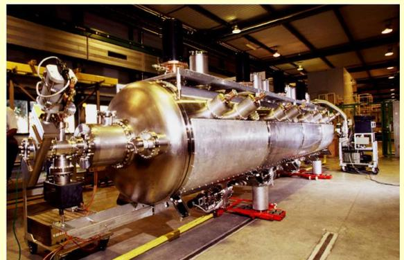
Superconducting cavities and cryomodules installed in the LHC, operating at an initial 7 TeV CM energy. At 400 MHz, 16 Nb-Cu cavities in 4 cryomodules provide 16 MV per beam and can deliver about 180 kW of beam power when needed. SRF cavities will help resolve the issue of transient beam loading by virtue of their low impedance and high cell voltage.
