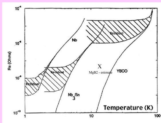
A comparison of superconductors Nb,  $\text{Nb}_3\text{Sn}$  YBCO and  $\text{MgB}_2$  at 1 GHz.
