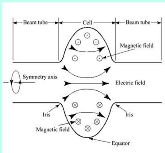
A single cell cavity shows electric and magnetic field lines for the accelerating mode as well as the location of the peak fields.
