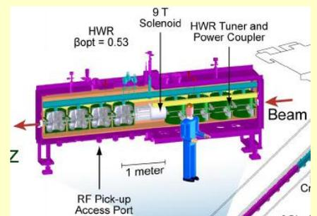
Cryomodule layouts for the QWR and HWR resonators. There will be 45 cryomodules in all.
