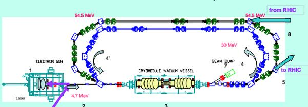
ERL for electron cooling the RHIC beam.
