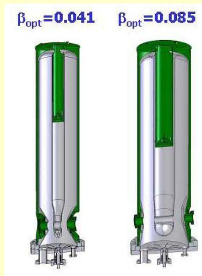
Quarter wave resonator designs for ReAccelerator3.
