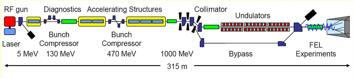
FLASH: One GeV linac for SASE FEL to 6.6 nm.
