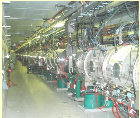
23 Cryomodules installed and operating at SNS.
