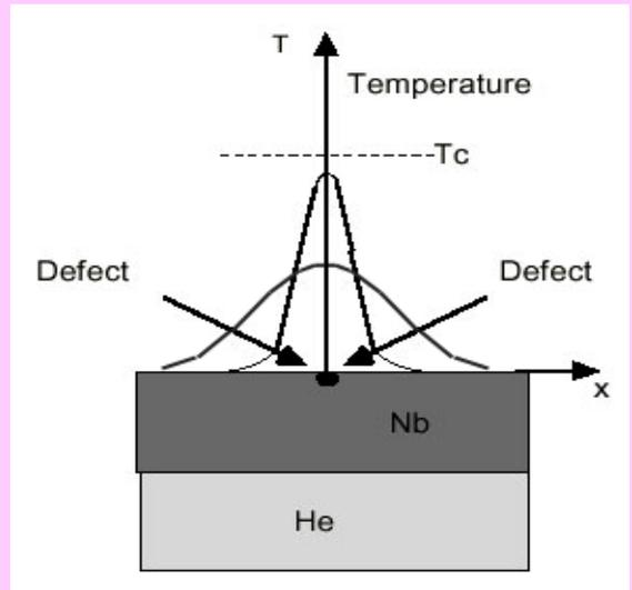
As the thermal conductivity improves, the defect and the niobium around it stay below the transition temperature. It becomes possible to raise the field further.
