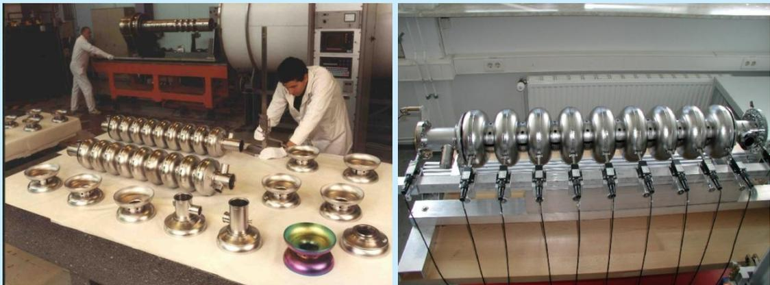
9-cell cavity fabrication and mechanical quality control at DESY.
