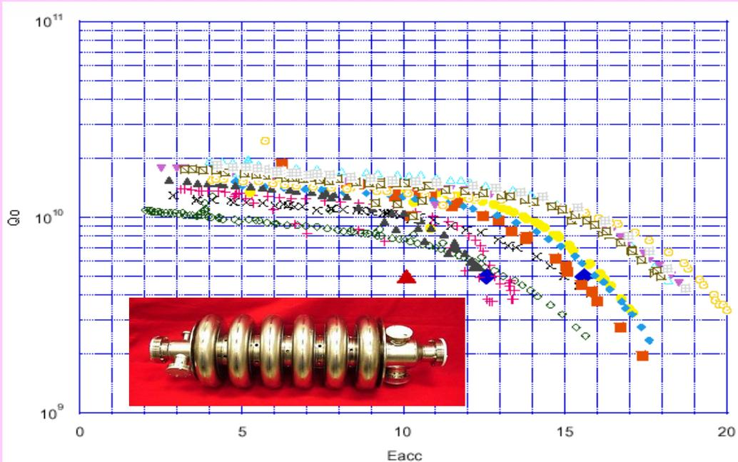
$\beta = 0.61$ , 805 MHz,  $E_{pk}/E_{acc} = 3.5$ , tested at JLAB.
