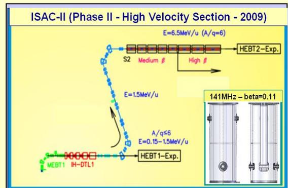
In the second stage (installation in 2010) another twenty cavities at  $\beta = 0.11$  (141MHz) will raise the final energy to 6.5 MeV/u, doubling the voltage gain of ISAC-II. The cavities will be housed in three cryomodules with six cavities in each of the first two modules and eight cavities in the third. Each cryomodule has one superconducting solenoid symmetrically placed in the cryomodule. Production of the cavities is with a Canadian company, PAVAC Industries of Richmond, B.C.
