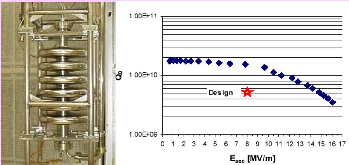
MSU,  $\beta = 0.49$ , 805 MHz, e-beam welded and tested at JLAB.
