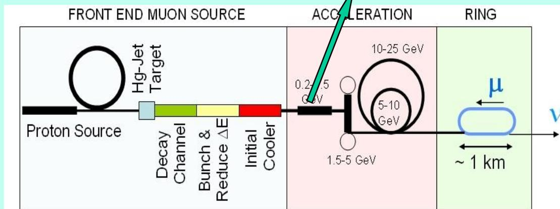
A generic neutrino factory from proton source to muon production, followed by cooling and acceleration. The demands on muon cooling are much reduced over that for a collider. In the final storage ring, muons decay to produce the desired intense neutrino beam.
