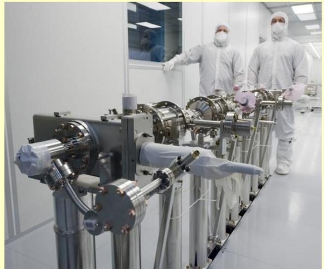
Clean Room assembly of four cavity package units at Fermilab.
