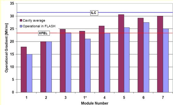
Evolution of cryomodule gradients over installation history. The bar chart compares linac and cavity acceptance test results. The average degradation is a few MV/m. Module 6 has only cavities prepared by the latest techniques of electropolishing and baking.
