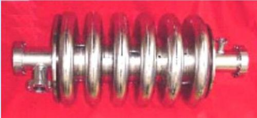
$\beta = 0.47$ , 800 MHz, 6-cell elliptical-cell (JLAB/MSU)
