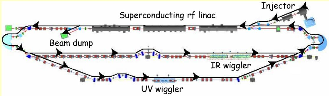
Layout of the Jlab IR FEL with UV upgrade. The FEL runs in the energy recovery mode. It comprises a 10 MeV injector, a linac consisting of three Jefferson Lab cryomodules generating a total of 80 to 160 MeV of energy gain, and a recirculator.
