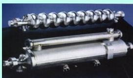
9-cell cavity and cryomodule for ILC.
