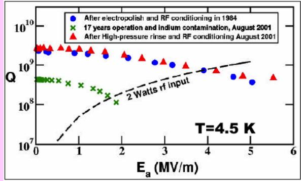
Argonne Split Ring Resonator, Frequency = 97 MHz,  $E_{pk} = 4.8$  Eacc,  $H_{pk} = 183$  Oe/MV/m. Performance improved substantially after high pressure rinsing.
