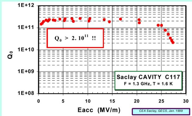
In some of the best performing cavities, Q values of  $10^{11}$  have been reached in 1.3 GHz single cell test cavities at 1.6 K and accelerating fields of 25 MV/m. The corresponding energy decay time is of the order of 10 seconds!
