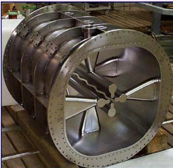
Superconducting RFQ for injector PIAVE at INFN.
