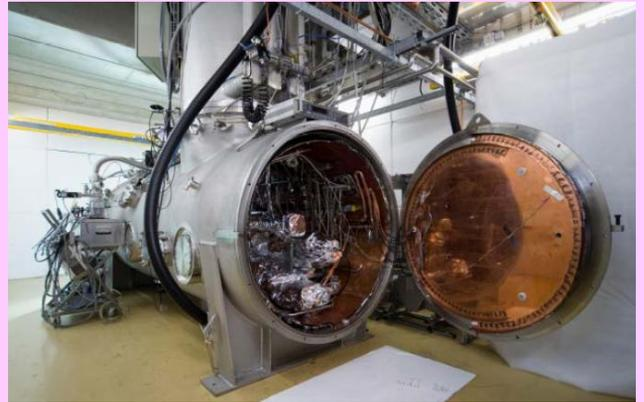
BESSY Cryomodule for testing 9-cell cavities equipped with coupler and tuner.
