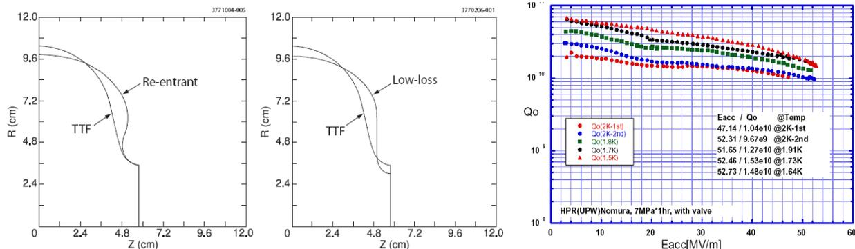
Comparison of cell profiles (a) TTF and Re-entrant shapes (b) TTF and Low-loss shapes.
