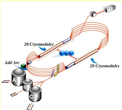
CEBAF is the largest SRF accelerator in operation in 2010. It has two 0.6 GeV linacs in the North and South tunnels, with 20 cryomodules each, and another 2¼ cryomodules in the injector making a total of 42¼ cryomodules. Each cryomodule has eight 5-cell cavities, making a total of 338 cavities. Having operated for more than 15 years it has accumulated more than 6 cryomodule-centuries of operating experience.
