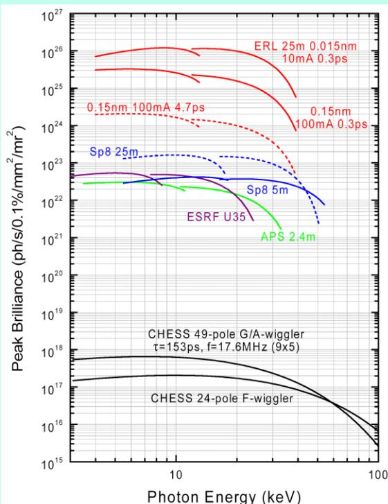
Cornell is proposing a synchrotron radiation light source as an extension to the CESR ring. The ERL will be driven by an energy recovering SRF linac operating at an energy of 5 GeV and an average current of 100 mA. While offering average photon flux comparable to storage rings, the proper parameters of an ERL can lead to higher peak brilliance, shorter pulses and a higher coherent fraction. The Cornell ERL will need 350 cavities and 60 cryomodules. KEK is proposing a similar 2.5 – 5 GeV ERL.
