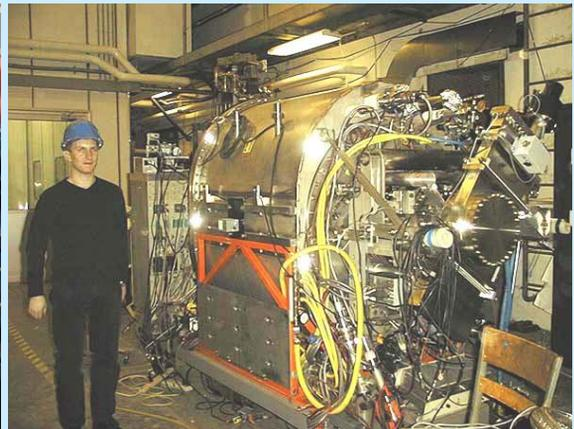
ERL injector and CESR Cryomodule assembly at Cornell.
