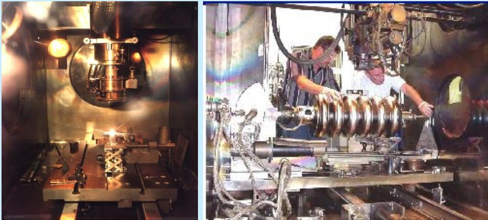
Electron beam welding at Cornell and JLAB.
