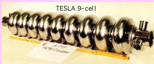
As field emission came under control in the late 1990's due to high pressure water rinsing and clean room assembly, gradients of 9-cell cavities improved steadily, as shown for 9-cell cavities between 1997 and 1999. By 2000, gradients consistently reached 25 - 30 MV/m.
