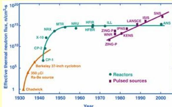
The highest intensity accelerator-based neutron sources in operation today are LANSCE at Los Alamos and ISIS at Rutherford Lab. The SNS at Oak Ridge National Lab is the first advanced pulsed spallation source with 1.4 MW of beam power at the target, upgradable to 5 MW. 6 Partner Labs: ANL, BNL, JLAB, LANL, LBNL, ORNL built SNS at ORNL in Oak Ridge Tennessee.
