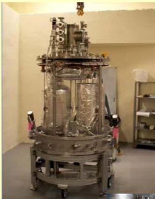
High beta cryomodule by Orsay.
