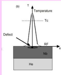
(Above) Temperature maps of a single cell cavity show spot heating as a precursor to large region of the cavity becoming normal conducting when the quench develops.
