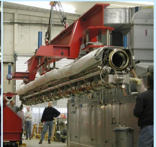
Cryomodule assembly at DESY.
