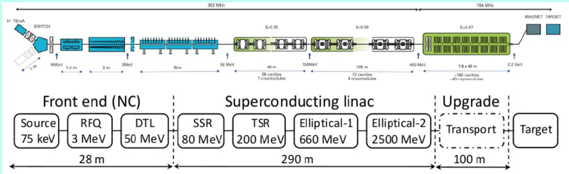
Schematic layout of ESS (European Spallation Source).
