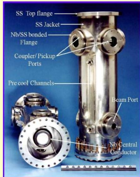
Completed resonator made from solid Nb and electron beam welding.
