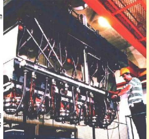
ATLAS Injector Cryomodule with inter-digital structures for particle velocities from 0.01c to 0.05 c (shown on left).
