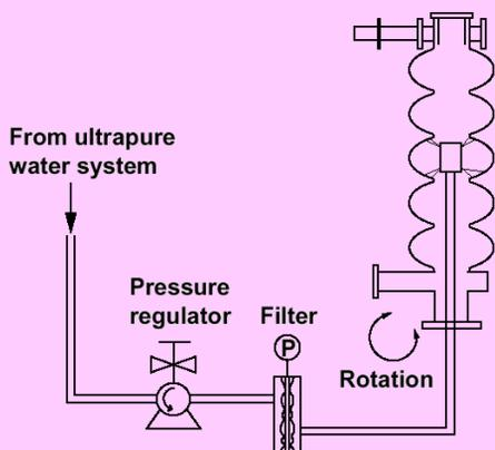
A jet of ultra pure water dislodges surface contaminants that normally resist removal with conventional rinsing procedures. The benefits of HPR in reducing field emission are well demonstrated in tests with multicell cavities that reach accelerating fields of 35 MV/m at DESY.
