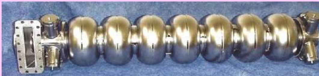
JLAB upgrade 7-cell Low-Loss cavity for lowering  $H_{pk}$ .
