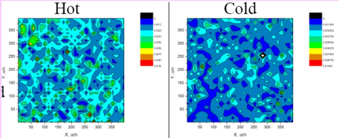
The hot samples show a high density of dislocations compared to the cold sample.
