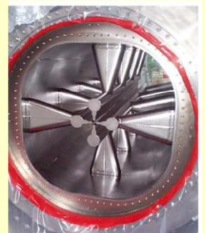
160 MHz medium beta PIAVE injector cryostat with Nb-Cu sputtered resonators. PIAVE extends the mass range of beams up to Uranium reaching 6 MeV/u of energy. In the very low  $\beta$  range from 0.01 to 0.05, the superconducting RFQ offers low power consumption for cw operation. Two structures delivered 4.7 MV in 2.13 m in PIAVE.
