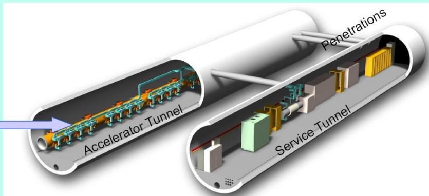
Two tunnel layout for the ILC, one for the accelerator and second for the RF sources and other services.
