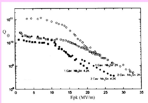
Performance of the best  $\text{Nb}_3\text{Sn}$  Cavity.
