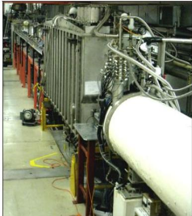
Energy upgrade cryomodule in the ATLAS tunnel.
