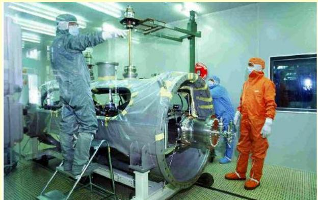
A pair of Nb/Cu single-cell HOM damped 352 MHz cavities, designed and built by a Saclay/CERN collaboration for SOLEIL and ESRF. The module (on the right) was high power tested at ESRF to Eacc of 7 MV/m and transferred 360 kW to 170 mA beam. Two modules have been installed and operated in SOLEIL to 300 mA beam current.
