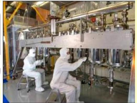
ATLAS energy upgrade cryomodule with seven  $\beta = 0.15$  structures (shown on left). The average accelerating gradient is 11.7 MV/m.
