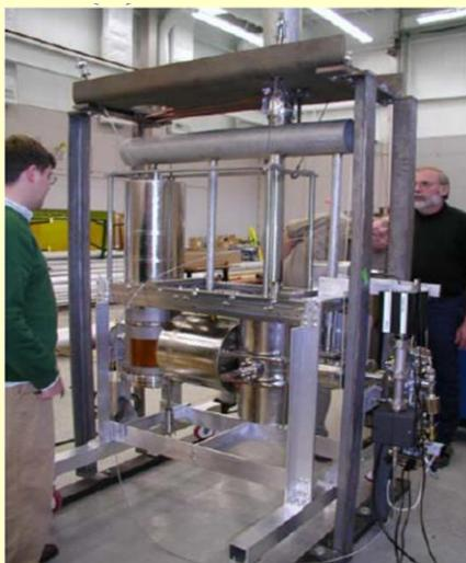
A prototype cryomodule housing a quarter-wave and a half-wave structure along with focusing magnets.
