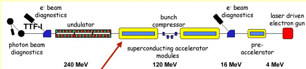
The first phase of the Tesla-Test-Facility (TTF).
