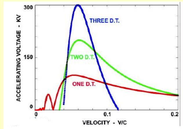
Non-relativistic ion beams require a broad velocity acceptance. The more drift tubes (D.T.) in a structure the more the total voltage gain, but at the cost of a smaller velocity range.
