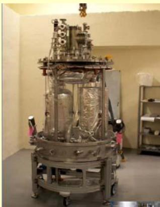
High beta cryomodule by Orsay.
