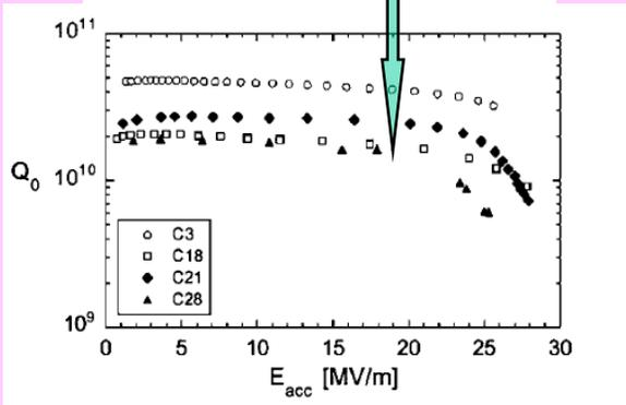
At 2 K, the BCS component of the surface resistance dominates the Q of  $2 \times 10^{10}$  so that lowering the temperature to 1.8 K improves Q to  $5 \times 10^{10}$ .
