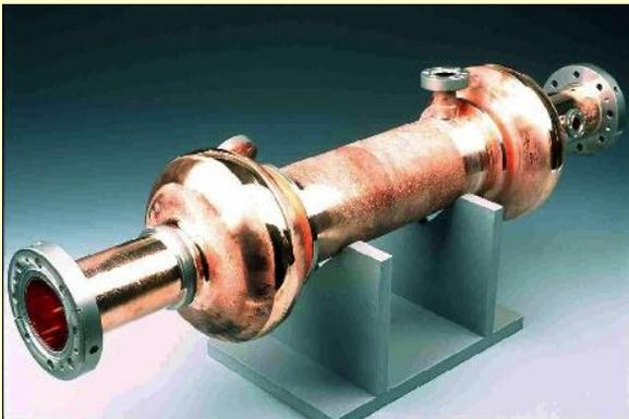
Prototype 3rd harmonic Cavity Built at CERN, Sputter coated with niobium.
