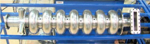
CEBAF upgrade 7-cell cavity has the Low-Loss shape to reduce dynamic heat load and stiffeners for operational stability.
