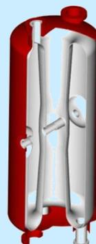
For the Half-Wave Resonator, suitable for  $\beta$  about 0.2, a coaxial transmission line, half wavelength long, resonates in the *TEM* mode. A drift tube is located in the middle of the hollow center conductor. The structure has two accelerating cells between the ends of the drift tube and beam hole openings located in the outer conductor of the coax. The structure period is  $\beta\lambda/2$ .
