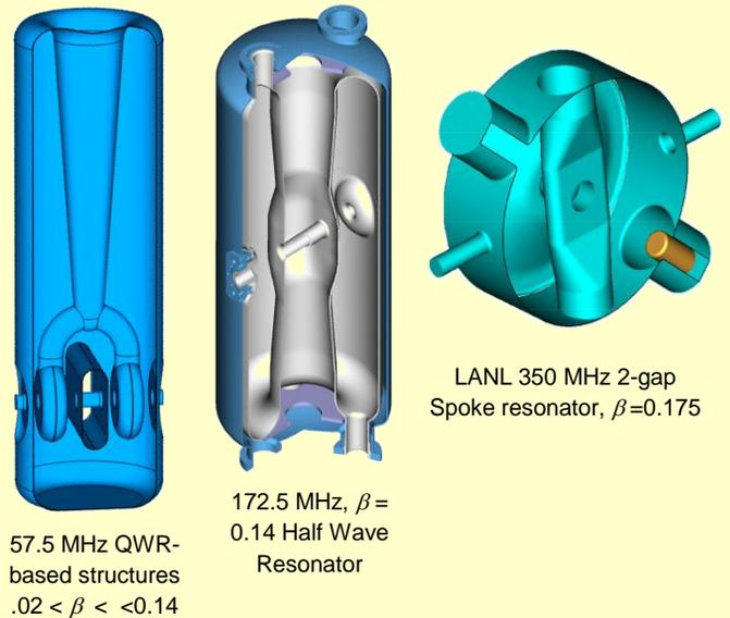
The peak surface to accelerating field ratios are significantly higher in the low-velocity structures. For a gradient of 1 MV/m, the peak electric field typically ranges from 4 to 6 MV/m (compared to 2 to 2.6 MV/m for  $\beta = 1$  structures) and the peak magnetic field ranges from 60 to 200 Oe (compared to 40 to 47 Oe for  $\beta = 1$  structures).
