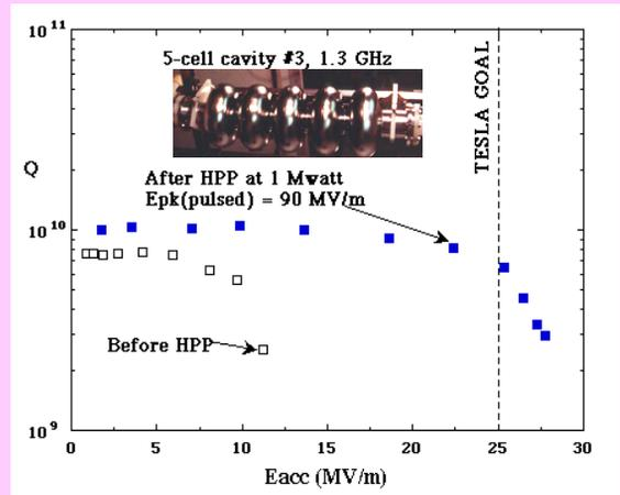
An example of "before-and-after" HPP. Here a cavity contaminated down to 10 MV/m improves with HPP to 28 MV/m.
