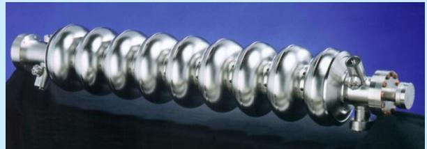
Photograph of a 9-cell, 1300 MHz, one-meter long accelerating structure with one input power coupling port at one end, and one HOM coupler at each end. It is used at FLASH and will be used in the European XFEL.
