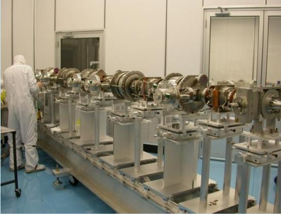
ERL-injector cavity string assembly at Cornell.
