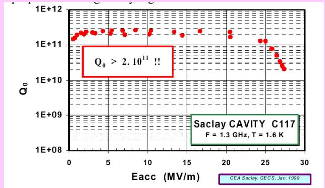
The world-record Q value is  $2 \times 10^{11}$  for a single cell 1.3 GHz cavity at 1.6 K and an ambient magnetic field less than 5 mGauss.
