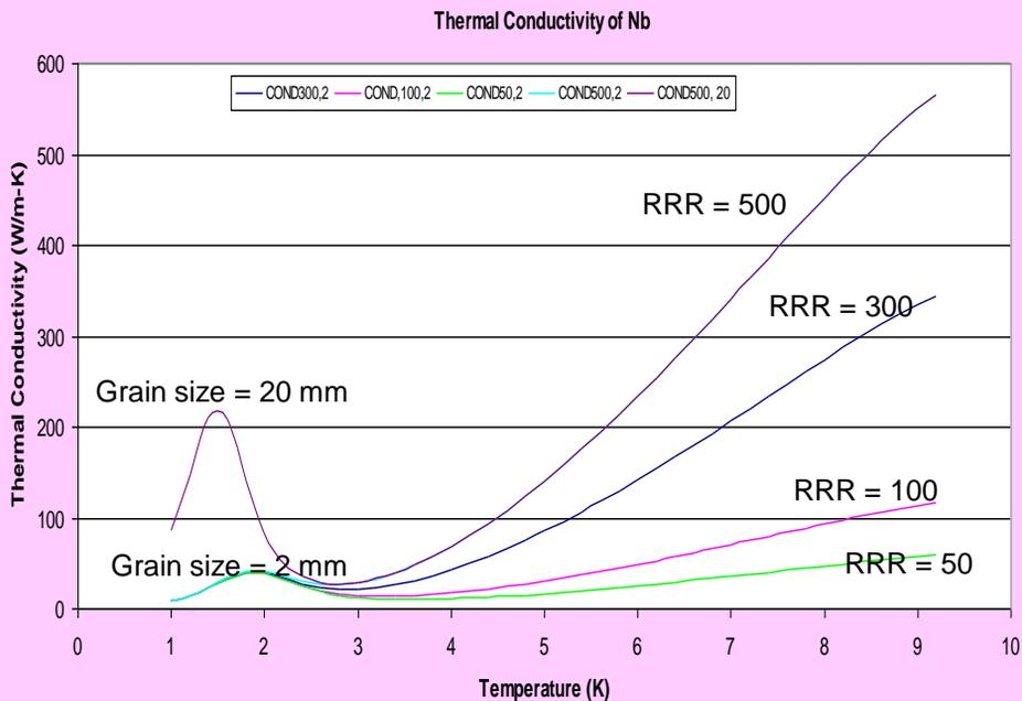
Temperature dependence of thermal conductivity for niobium of various purities, as characterized by the RRR. The thermal conductivity of niobium decreases rapidly with temperature below  $T_c$ , because electrons, the dominant heat carriers, rapidly freeze out into Cooper pairs. Below 2 K there is a phonon conductivity peak which increases sharply with grain size. The phonon peak does not help stabilize defects against quench because the temperature around the defect is well above 2K.
