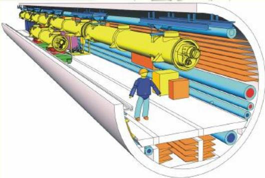
The European XFEL main linac tunnel cross section, 5.2 m diameter.
