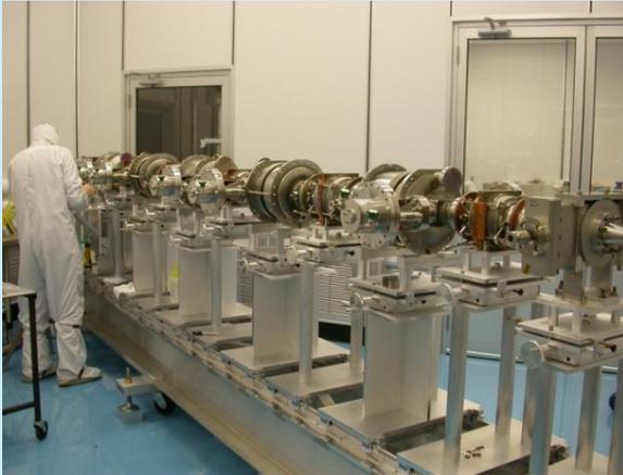
ERL-injector cavity string assembly at Cornell.
