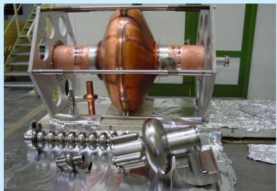
A variety of superconducting cavities for accelerating velocity-of-light particles. In the foreground (left) is the 9-cell cavity and (right) a CESR 500 MHz cavity together with a 1/3-scale version of the latter. In the background the large 200 MHz Nb-Cu cavity dominates. With a few micron layer of niobium sputtered on the inside, the cavity was developed by a Cornell/CERN collaboration for future muon accelerators and the neutrino factory.
