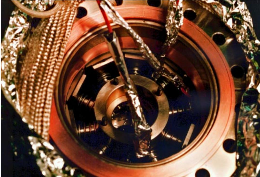
**Figure 5.3.** Tiles being soldered to one unit of the ferrite structure. The upper-most of four “Mini-Tribendis Wheels” (used to clamp the tiles in place while they are being soldered) is visible.
