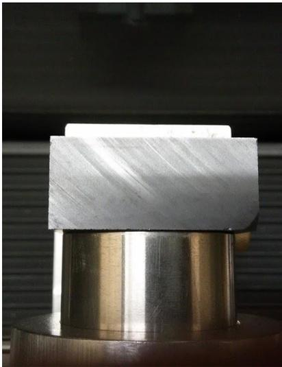
Figure 12(a): Top view of Asymmetric Si 7 5 3 Crystal 1 during Laue diffraction
