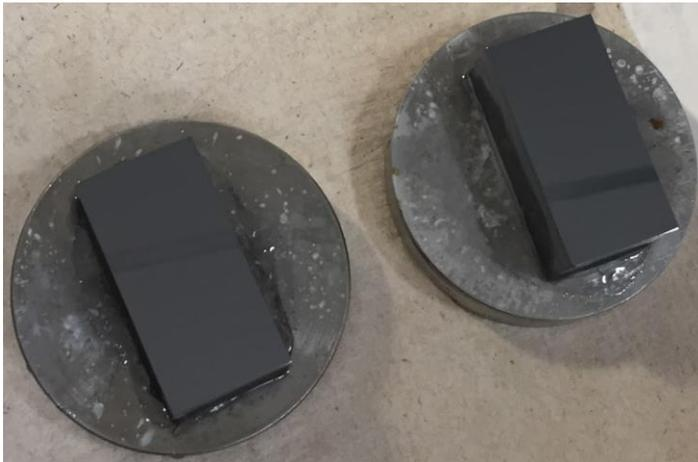
**Figure 8:** Asymmetric Si 7 5 3 Crystal 1 and 2 after  $\text{Al}_2\text{O}_3$  slurry
