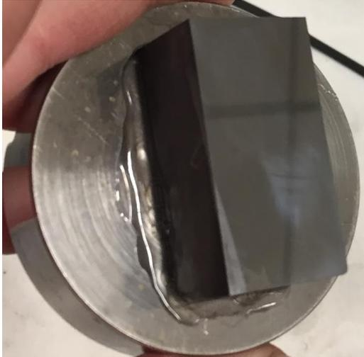
**Figure 7(b):** Asymmetric Si 7 5 3 Crystal 2 after polishing wheel, Reflective except for left edge, some scratches present
