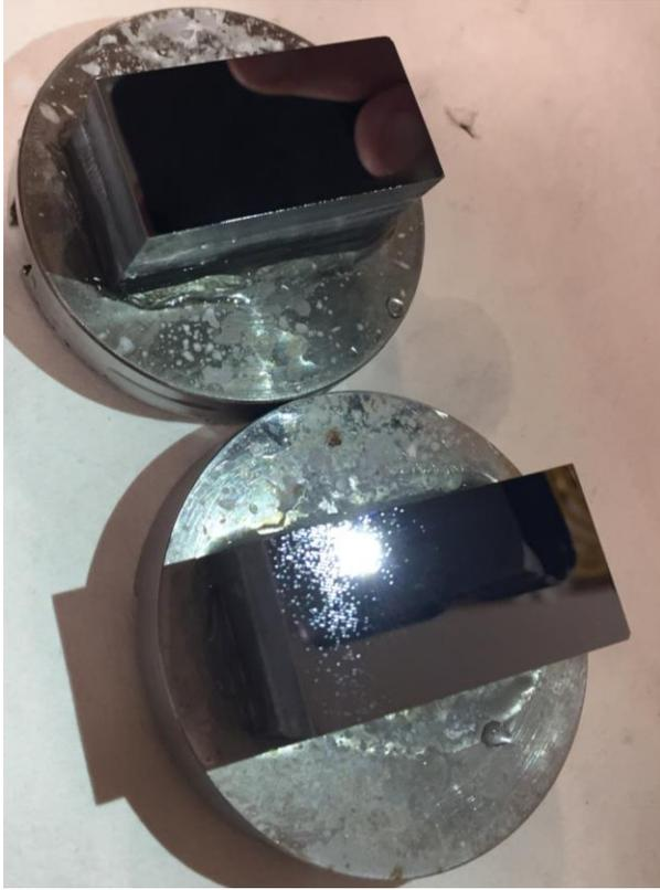
**Figure 9:** Asymmetric Si 7 5 3 Crystal 1 and 2 after Silica slurry, Small scratch removal
