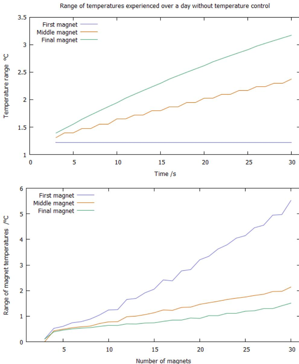
Figure 6: a) The temperature variation of magnets over 1 day, with no cooler control
