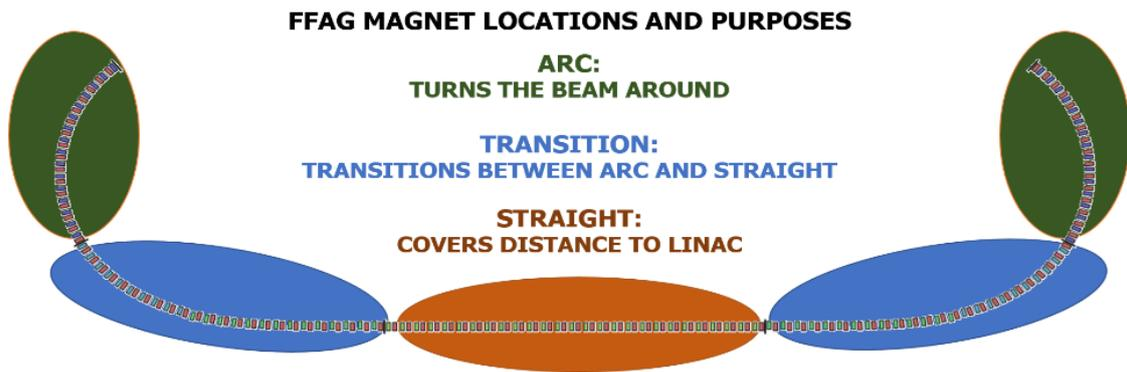
Figure 1: The sets of FFAG magnets, forming the return loop of the accelerator. Note that the total circumference of CBETA is 79.1 metres.
