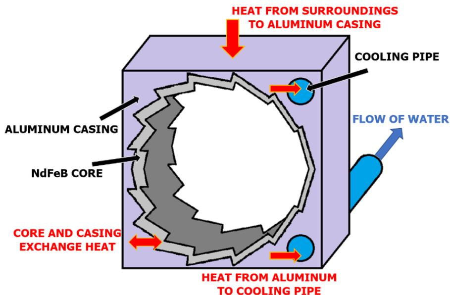
Figure 2: A summary of the continuous thermal transport processes in each FFAG magnet (NdFeB is the Neodymium-Iron-Boron magnet core). Note that this is not to scale: for magnet dimensions, see appendix.
