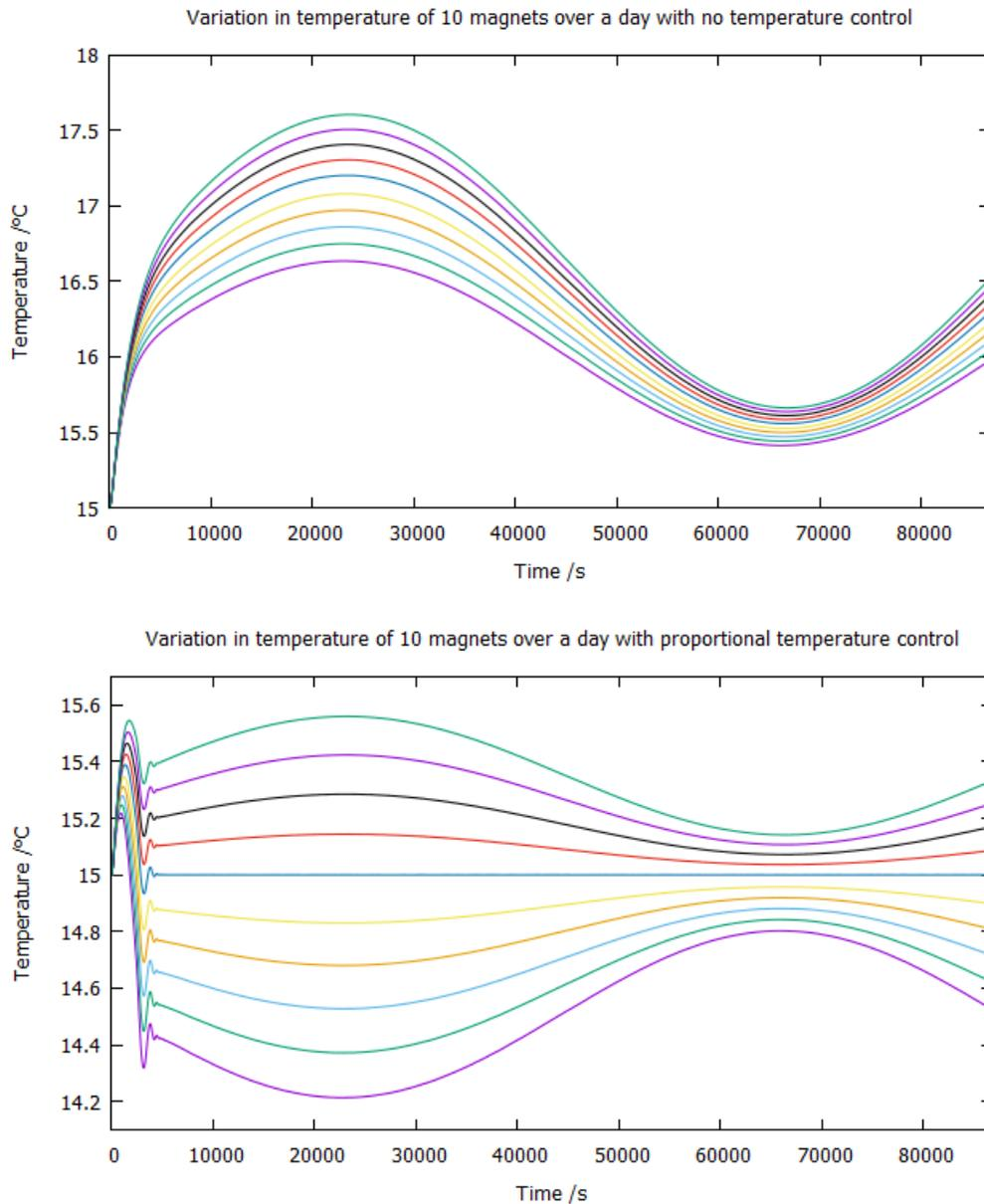
Figure 3: a) Temperature variation in 10 magnets over 1 day, with no cooler control
