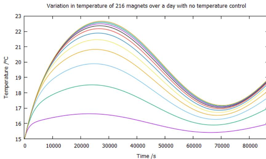
Figure 4: Temperature variation in 216 magnets over 1 day, with no cooler control
