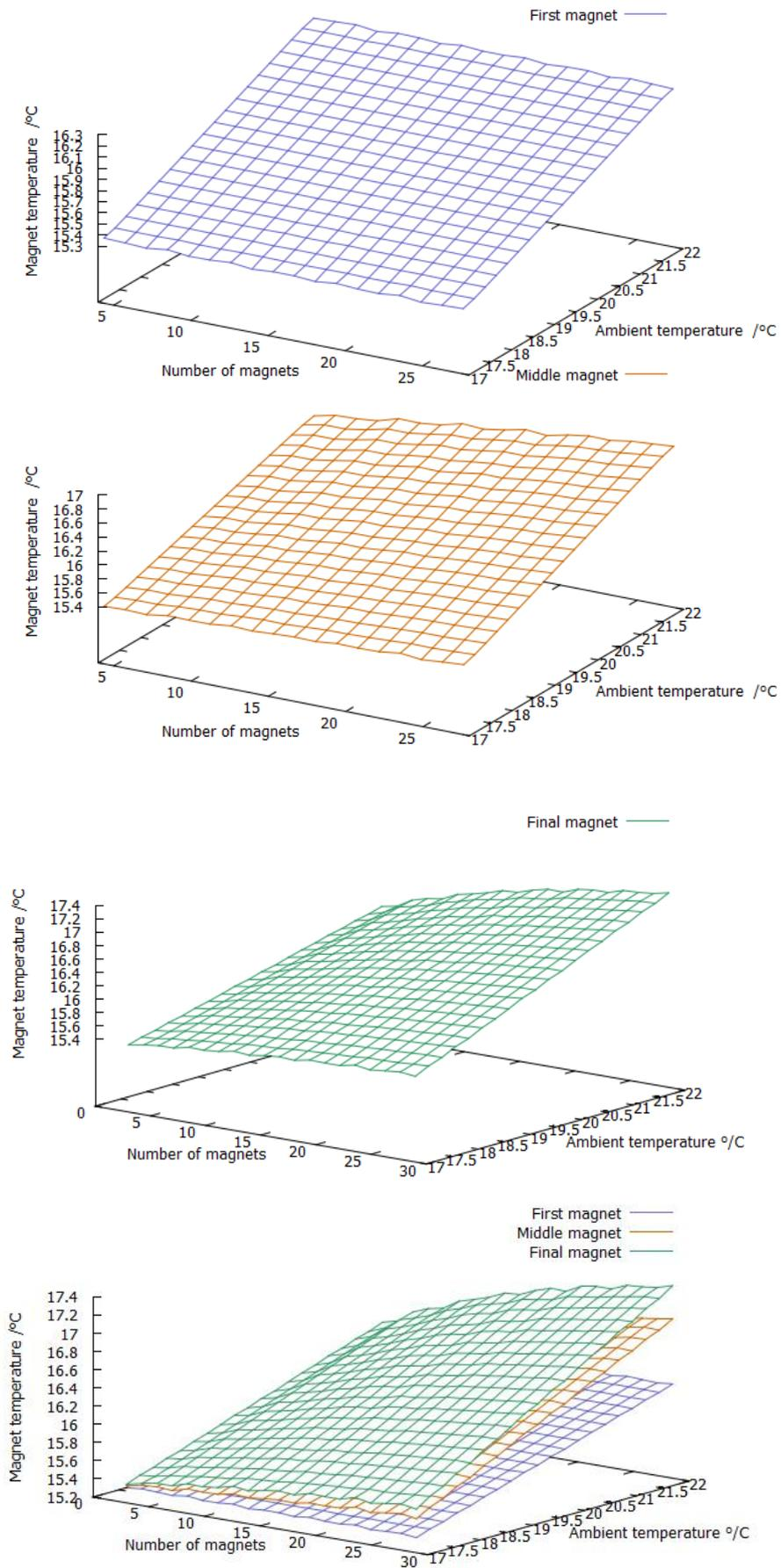
Figure 5: variation in stable temperature with number of magnets, measured for three different magnets in the ‘circuit’. The measured magnet is labelled by color in the top right of each diagram.
