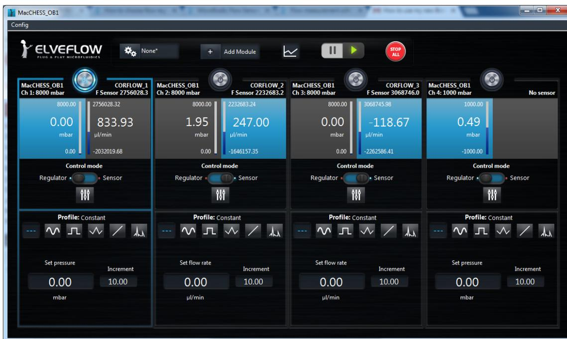
Figure 18 - The Elveflow software interface to the OB1 pressure controller.
