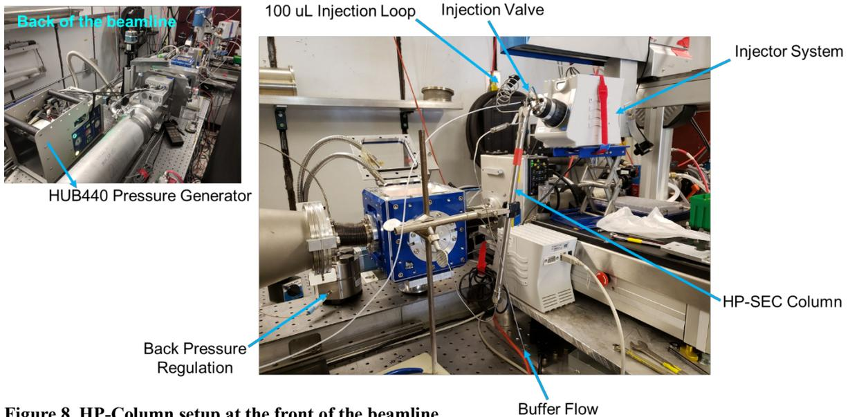
**Figure 8. HP-Column setup at the front of the beamline**
