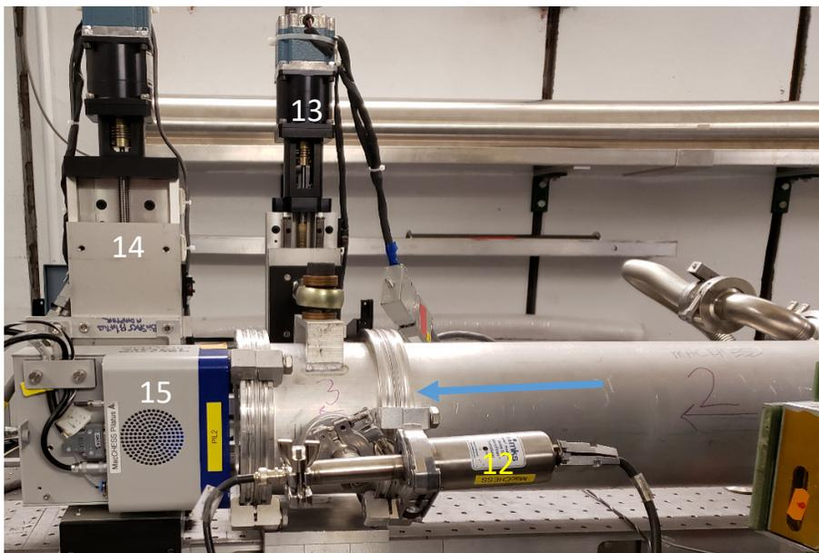
**Figure 5.** The rightmost selection of the front 1D7A1 beamline; #12 is a MicroPirani Transducer connecting to a vacuum gauge (not visible in Figure 5); #13 is a bsx/bsz motor of beamstop; #14 is a ccdx/ccdz motor of #15, Pilatus 100K detector, to detect scatters of x-ray beams. Vacuum of the flight path must be equal to 10 mTorr or lower to get the best quality of scattering.
