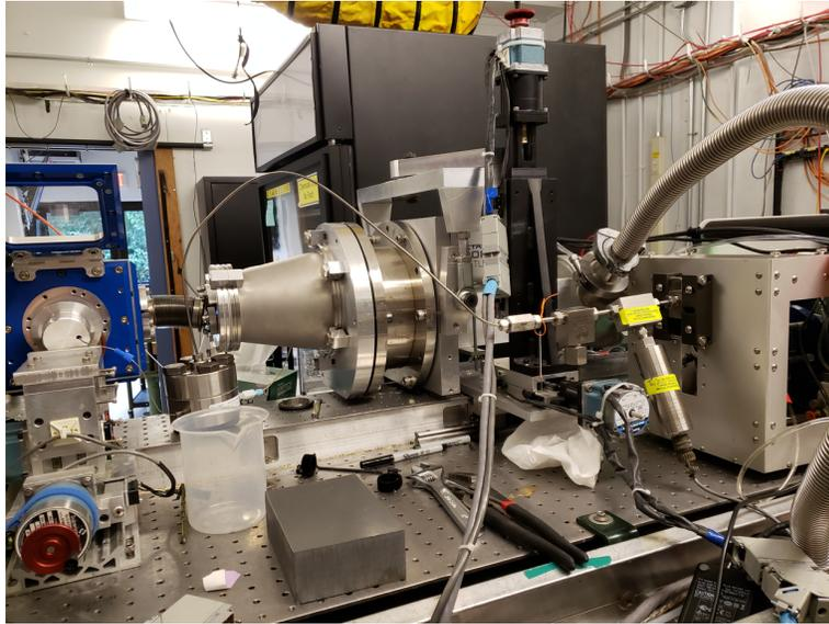
Figure 9. HP-Column and Pressure Generator set-up at the behind of the beamline
