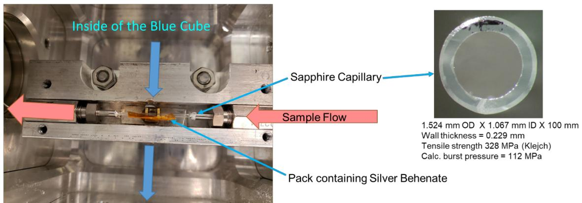
Figure 10. Inside of the blue cube and sapphire capillary setup
