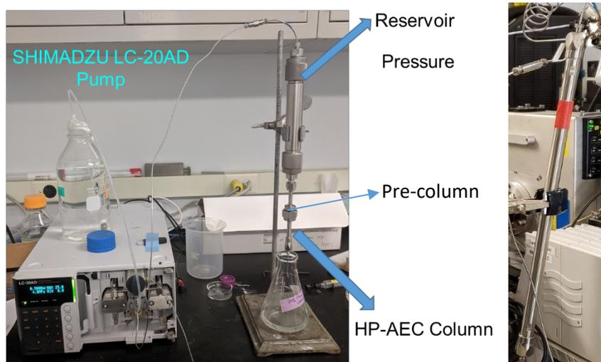
**Figure 11. Packing the High-Pressure set-up (left) and HP-SEC column (right)**
