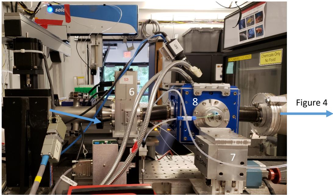
**Figure 3.** The middle selection of the behind 1D7A1 beamline. #6 is a guard slit  $S_3$  (to clean up “parasite” scatter”); #7 is a backside of X-Z stage to support and move #8, a blue cube (detailed in Figure 10.)
