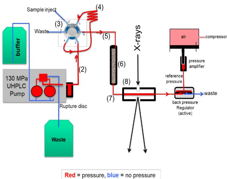
**Figure 6. Simplified Diagram of the Sample and Buffer Flow under Pressure.** 2# Metal tube; 3# IDEX injection valve; 4# 100 microliter loop; 5# metal tube; 6# high-pressure column; 7# metal tube; and 8# sapphire capillary (inside of the blue cube).
