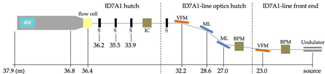
**Figure 1. Simplified Diagram of the BIO-SAXS Beamline inside of the 1D7A1 hutches**
