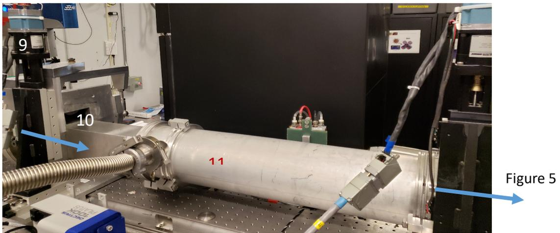
**Figure 4.** The middle-rightmost selection of the behind 1D7A1 beamline; #9 is F11x/F11z motor, to move the upstream end of the pipe; #10 is a vacuum window (must be sealed with plastic paper and epoxy-based glue); and #11 is a flight path (pipe).
