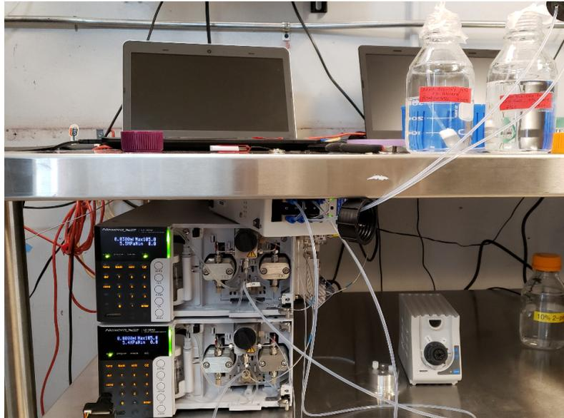
**Figure 7. Nexera X2 – LC-30AD pumps setup (two pumps were required for AEC experiments - more details at bottom)**
