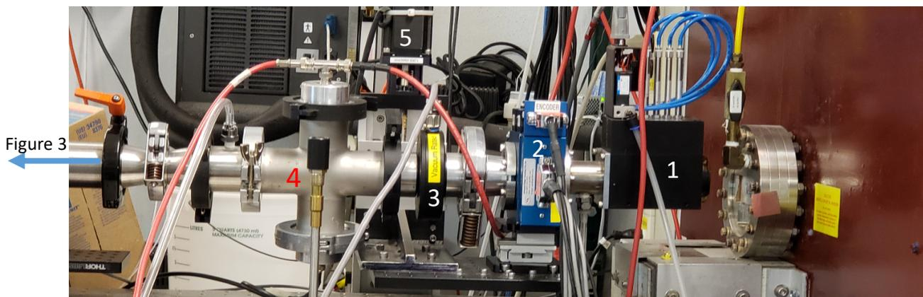
**Figure 2. The leftmost selection of the front 1D7A1 beamline (next to G-Cave x-ray micro-window.)** The section #1 is an attenuation; #2 is a controllable S4 slit (and is also movable using #5, an upstream motor); #3 is a vacuum rated shutter; and #4 is an ion-chamber (I<sub>4</sub>), a measurement of x-ray intensity.
