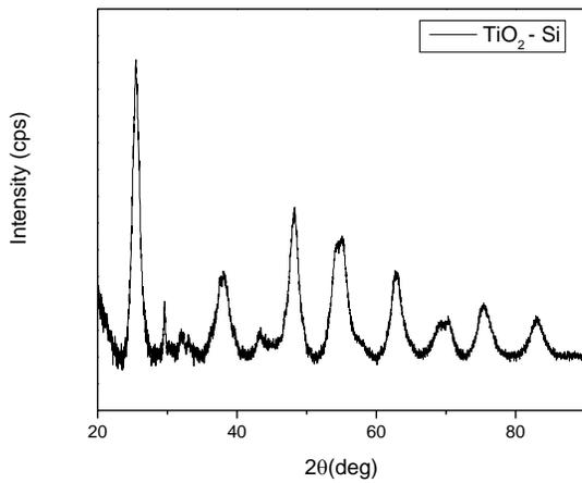
**Figure 2.** X-ray diffraction of Titanium dioxide doped with silicon. The obtained pattern is consistent with the anatase phase of  $\text{TiO}_2$ .
