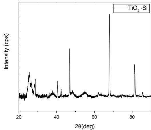
**Figure 3.** X-ray diffraction of Titanium dioxide doped with silicon after grinding.
