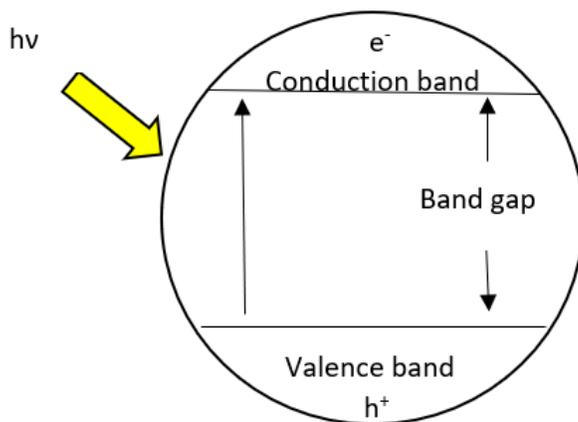
**Figure a.** Schematic illustration of photo-generation of charge carriers in a photocatalyst.
