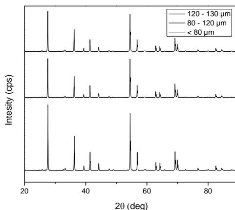
**Figure 1.** X- ray diffraction of nano- $\text{TiO}_2$  ( $<80\ \mu\text{m}$ ,  $80\ \mu\text{m}$  -  $120\ \mu\text{m}$ ,  $120\ \mu\text{m}$ -  $130\ \mu\text{m}$ ) in rutile phase.
