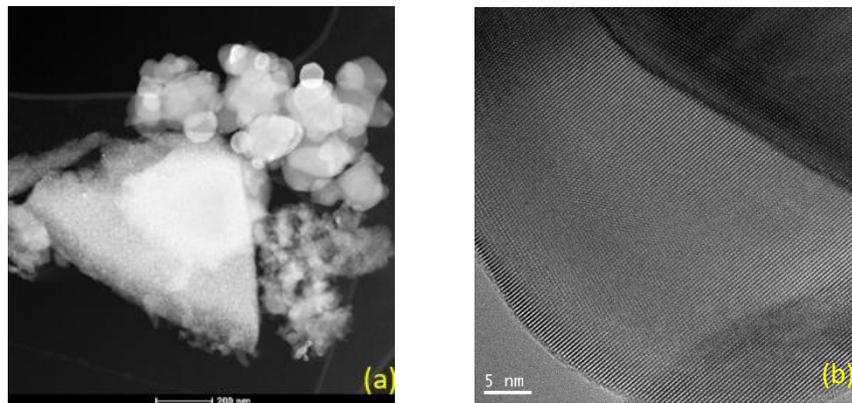
**Figure 4.** TEM images of (a) Si doped  $\text{TiO}_2$  nanoparticles (b) High resolution TEM images of Si doped  $\text{TiO}_2$  nanoparticles.
