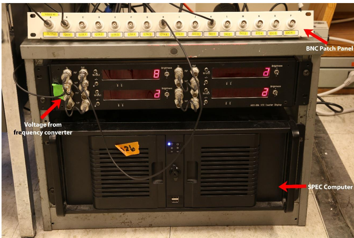
Appendix Figure 1: SPEC computer (labeled connections)
