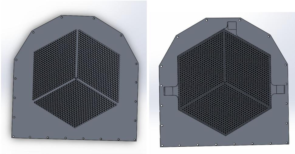
*Figure 5 : Feedhorn Block, Designed by using Solidworks*
