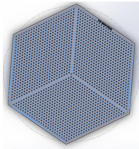
*Figure 4: Hexagonal Detector Wafer Designed by Using Solidworks*
