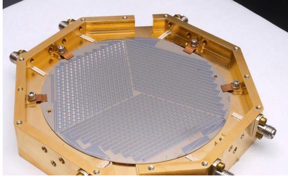
*Figure 1: microwave kinetic inductance detectors array*
