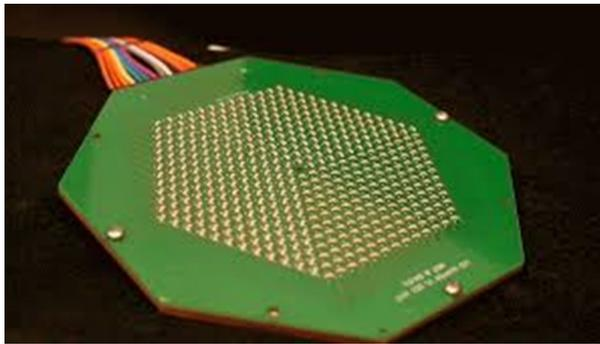
*Figure 2: Hexagonal cryogenic wafer mapper based on light emitting diodes (LED).*
