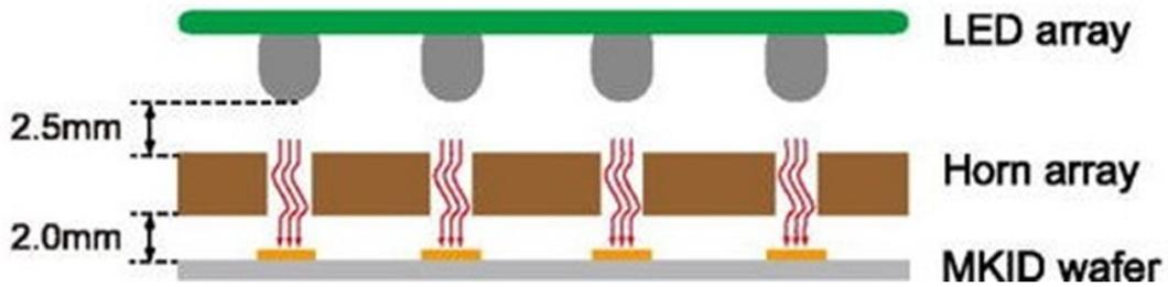
*Figure 3: The Assembly Alignment*
