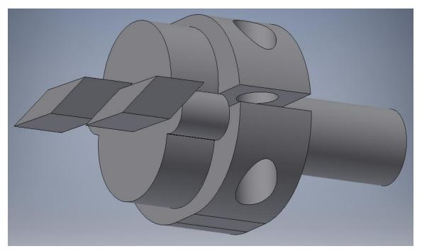
Final assembly of the galvanometer-based fast X-ray shutter. All the design process was done using a computer aided design (CAD) program Autodesk Inventor.
