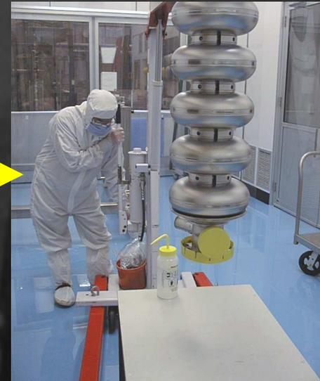
Cool down and test the performance of the cavity
