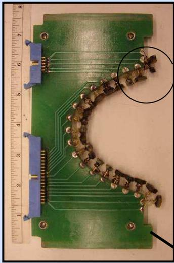
756 Allen Bradley copper resistors are used to obtain temperature map (~1 resistor per square cm)
