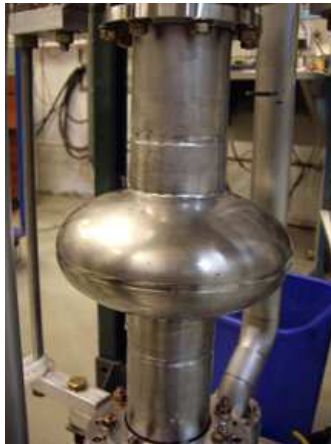
FIG. 1: Picture of a 1.5Ghz cavity mounted to a test stand
