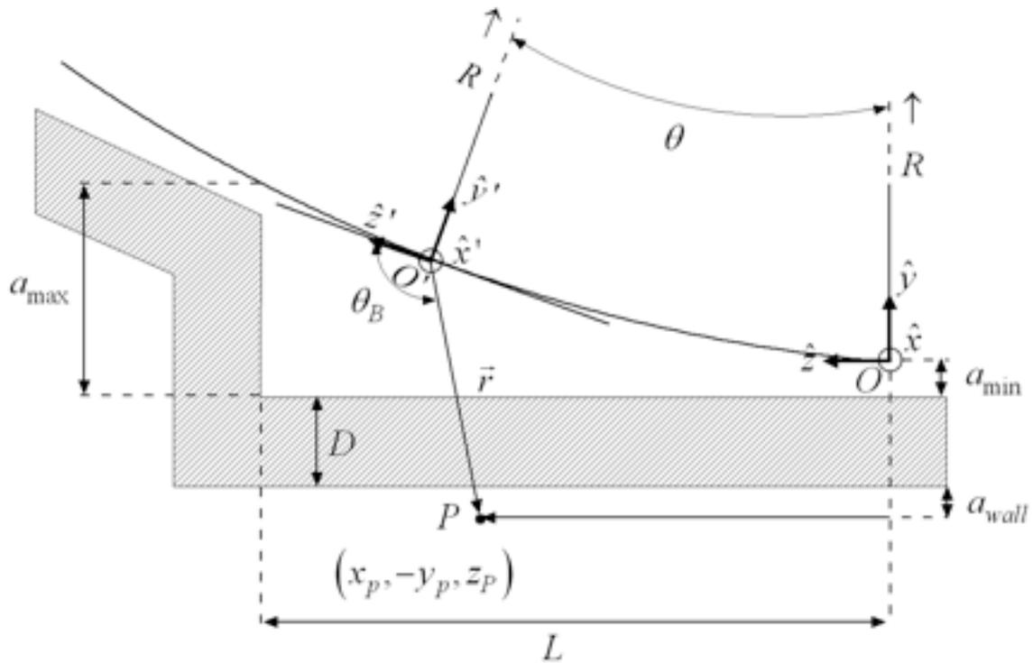
Figure 5: ERL ratchet shielding wall geometry.
