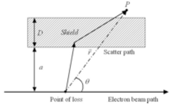
Figure 4: Indirect path of radiation.
