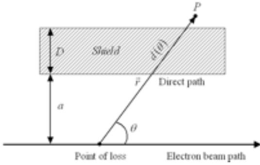
Figure 3: Straight line path of radiation.
