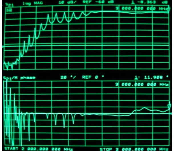
FIG. 3: Network analyzer data for the phase shifts caused by a Lexan plastic dielectric in the physical conductor. The amplitude for each frequency is shown on top at 10dBm per division; the corresponding phase shifts are shown on the bottom at 20° per division.
