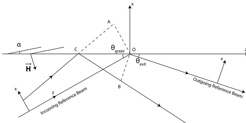
Figure 1: Ray diagram showing how the 3 sets of basis vectors are defined. The  $y$ -axis for all 3 of the bases are defined to point out of the paper. In this diagram, all lines and rays are in the plane of the paper, except for those defined by the off-axis photons which may have a  $y'$  component. This means that the points A, B, C do not necessarily lie in the  $x-z$  plane.
