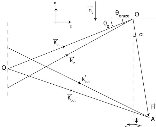
Figure 2: Diagram showing the construction in reciprocal space to find the directions of the center of reflection. All points shown in the diagram are in the plane of the paper, except for the point A. The y-axis points out of the plane of the paper.
