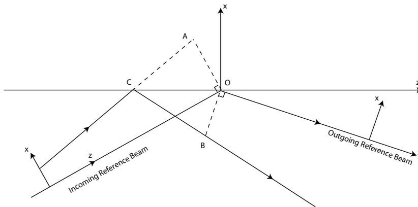
Figure 3: Diagram showing reference and off-axis rays in real space. In this diagram, only the incoming reference beam has to be in the plane of the paper; points A,B,C are not necessarily in the x-z plane.
