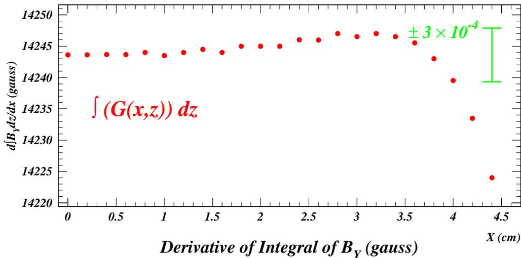
⇒ Integrated gradient uniformity at 4.7 kA:  $\pm 3 \times 10^{-4}$  out to 4.0 cm
