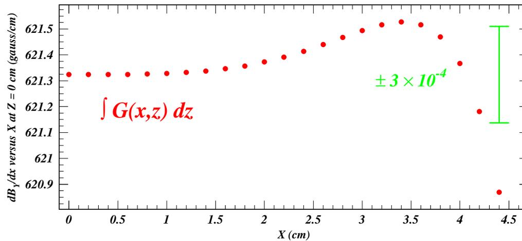
⇒ Integrated gradient uniformity at 14 kA:  $\pm 3 \times 10^{-4}$  out to 3.8 cm
