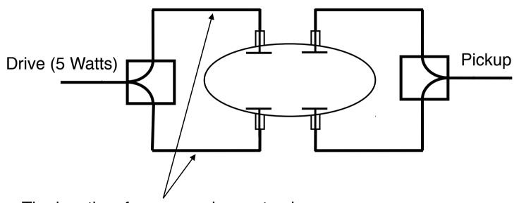
The lengths of coax are chosen to give 180° phase shift at the drive frequency.
