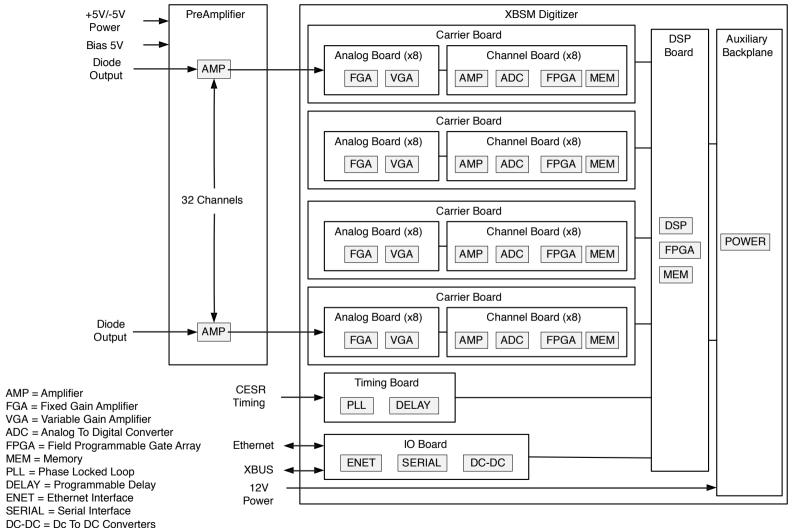
DSP = Digital Signal Processor POWER = Power Distribution
