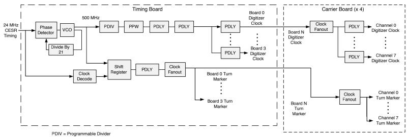
PPW = Programmable Pulse Width PDLY = Programmable Delay
