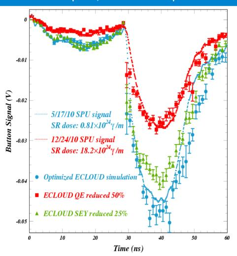
Shielded pickup signals measured in an amorphous-carbon-coated chamber in May (blue dotted line) and December (red dotted line) of 2010 for two bunches carrying  $4.8 \times 10^{10}$  5.3 GeV positrons 28 ns apart. The synchrotron radiation dose increased by a factor of twenty during this time interval. The ECLOUD model optimized for the May data is shown as blue circles, the error bars showing the model statistical uncertainties.
