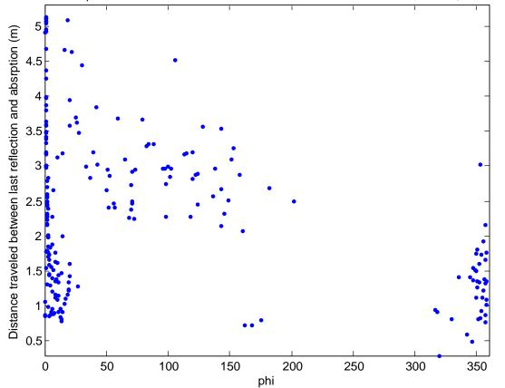
Distance each photon traveled between its last reflection and where it was absorbed, smooth wall
