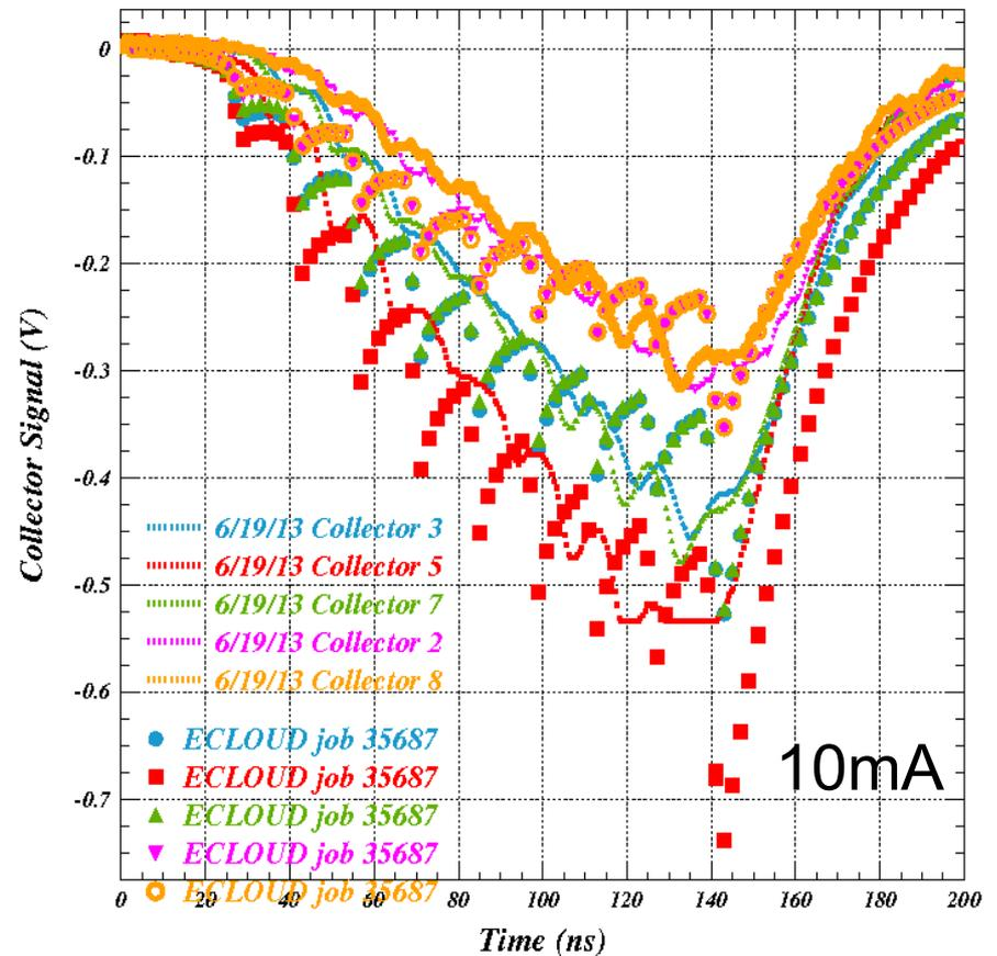
Our hope was to design an angular acceptance scheme that would be robust for changes in the bunch current away from the 8mA/bunch for which it was designed. Here we see that the model handles an increase in bunch current to 10mA/bunch well, maintaining both the relative sizes as well as the overall size and timing. Lowering the current to 6 mA however, we see that the model breaks down, with a size that is ~20% too large across all collectors.
