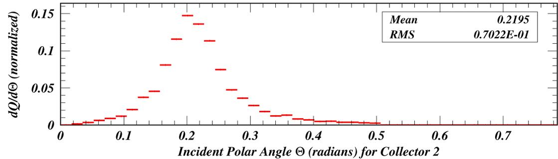
Each successive collector has a peak angular acceptance  $\sim .05$  radians different than the previous.
