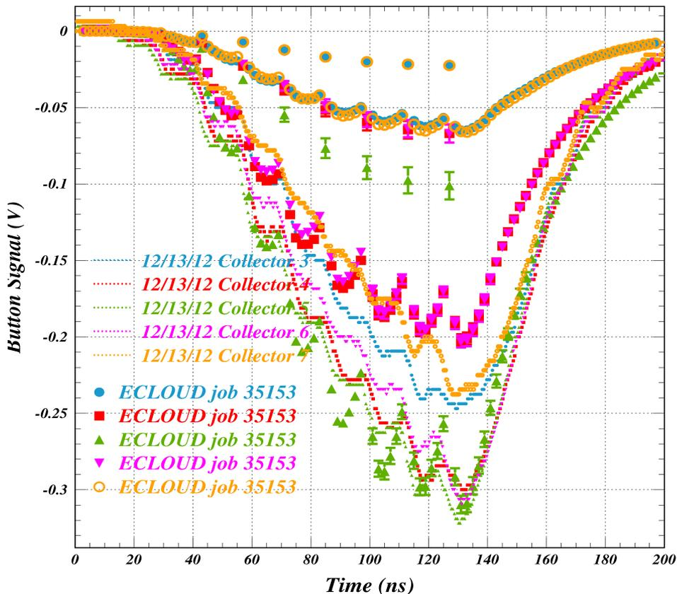
Using the angular acceptance function calculated separately by Joe Calvey (shown at left), the TR\_RFA model shows good agreement for the central collector, number 5, only (at right, presented on 10 April, 2013). The signals modeled for the outside collectors are considerably smaller than we need.
