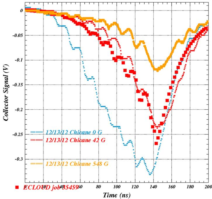
Chicane Scan: 5.3 GeV e+ 8 mA/bunch TR\_RFA04 Collector 5 Smooth Al
