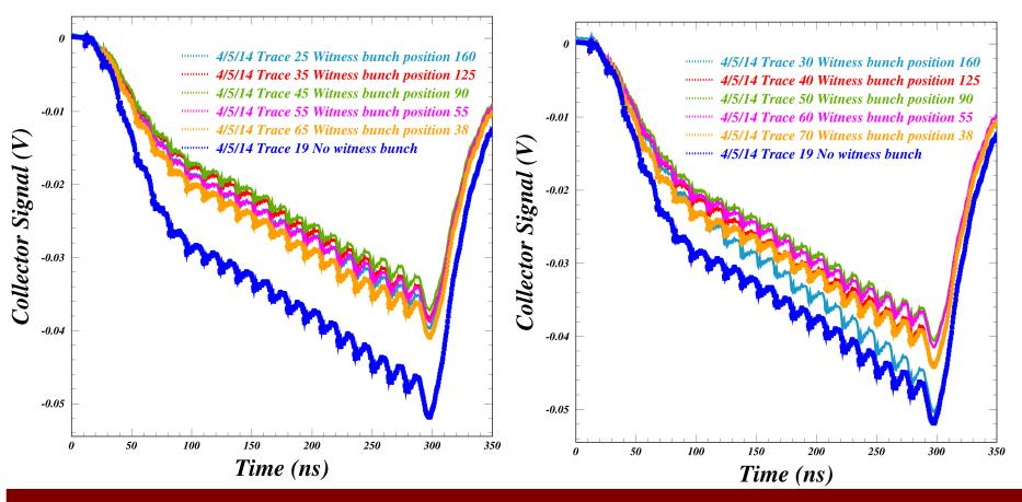
The clearing effect depends only weakly on position. A single bunch is more effective than a 6-bunch clearing train. The optimal position is about halfway around the ring.
