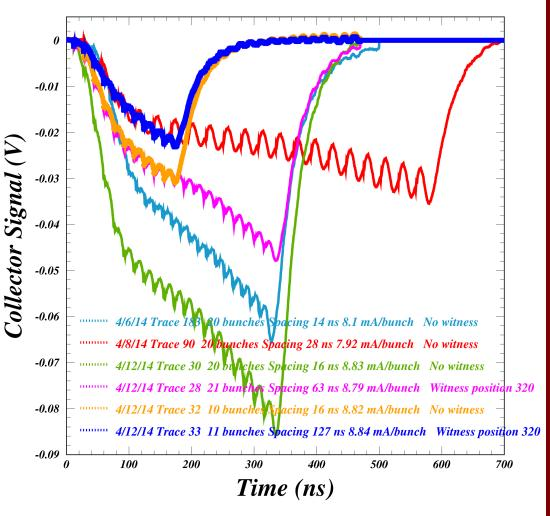
I) The signal from the 20-bunch train with 28-ns spacing is about half of that of the 14ns spaced train. The trapped cloud which contributes to the signal is cleared by the first three bunches rather than the first six. Will the trend hold for spacings between 14 and 28 ns?
