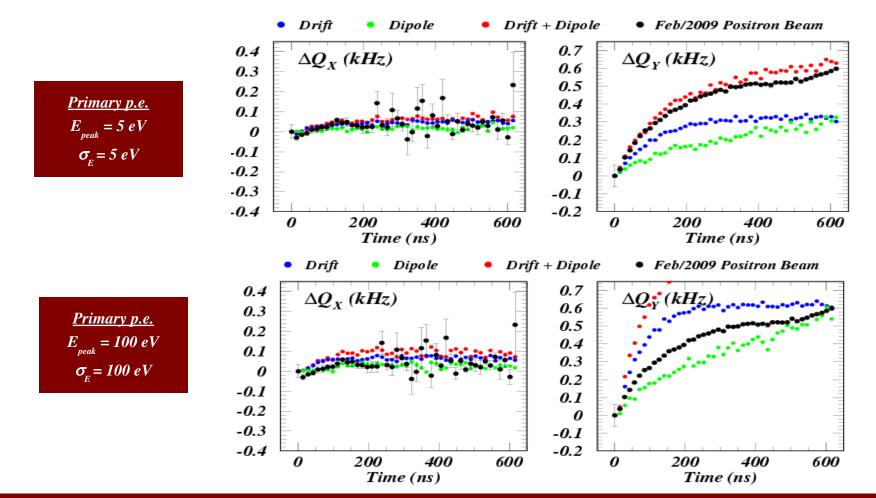
The consequences of the photoelectron energy spectrum are exaggerated here, because it is too hard on average. Nonetheless, we can expect the drift region contribution to be enhanced relative to that of the dipole regions.
