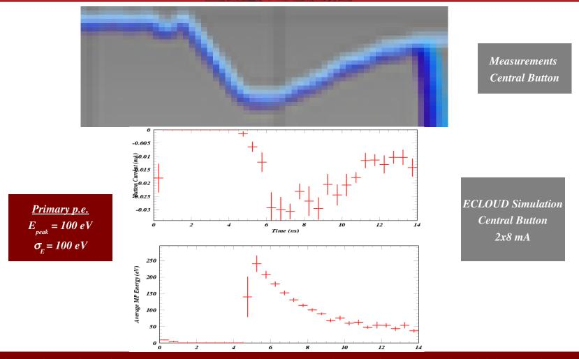
For the electron beam, the earliest energy is 250 eV, rather than 900 eV. This is too low to correctly model the arrival time.
