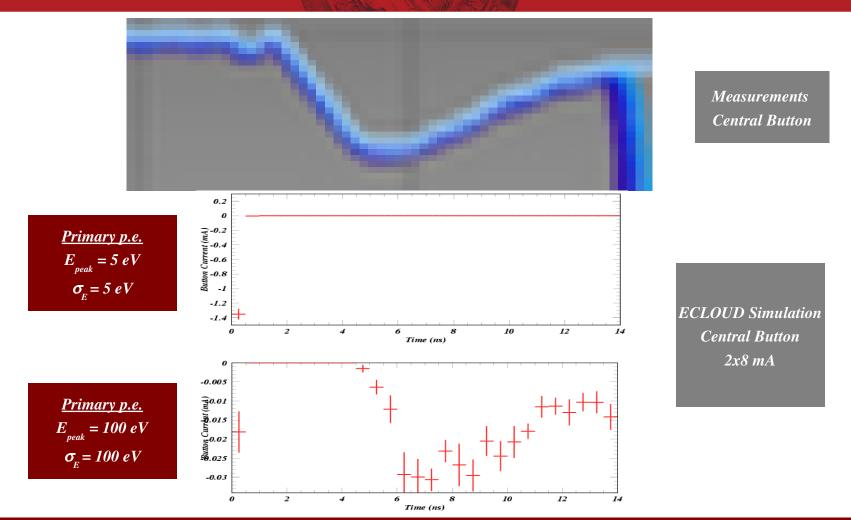
The cloud particles produced on the floor must overcome the potential barrier of the electron beam to reach the ceiling. Their arrival time is very sensitive to the high end of the energy spectrum and to the production angular distribution. For example, the signal arrives at 12 ns for  $E_{peak} = 40 \text{ eV}$   $\sigma_E = 20 \text{ eV}$ , rather than at 5 ns for  $E_{peak} = 100 \text{ eV}$   $\sigma_E = 100 \text{ eV}$ .
