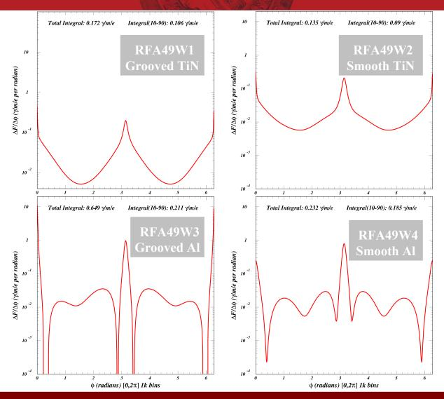
Synrad3D calculates quite different photon rates and distributions in the four TR-RFA chambers.
