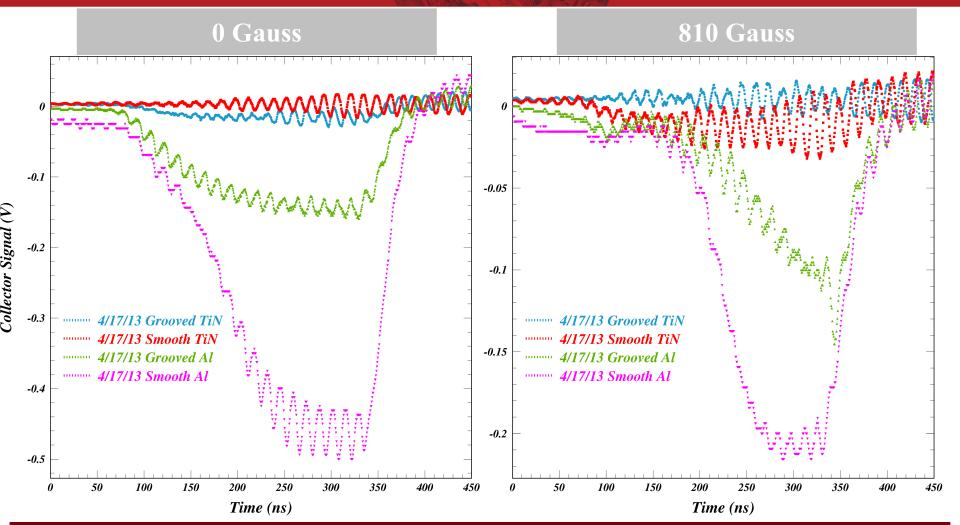
In spite of beam noise and ringing, the reduction of cloud with TiN grooves is clear.
