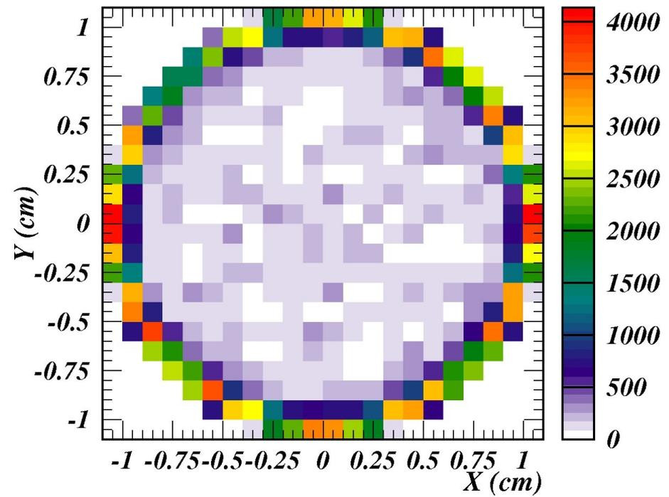
The quadrupole symmetry is broken by the rotated longitudinal magnetic field.
