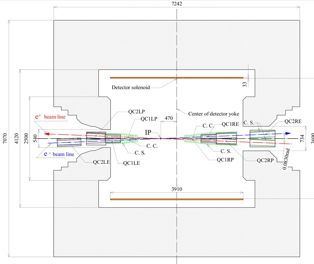
The BELLE-II solenoid is offset by 470 mm relative to the IP in the flight direction of the 7-GeV electron beam. The final-focus quadrupole QC1RP for the 4-GeV positron beam is in the region of uniform solenoid field.
