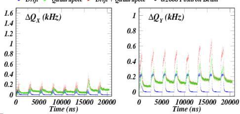
The tune shifts calculated from the field gradients at the center of the vacuum chamber show turn-to-turn buildup behavior similar to that for those calculated with offset beams.
