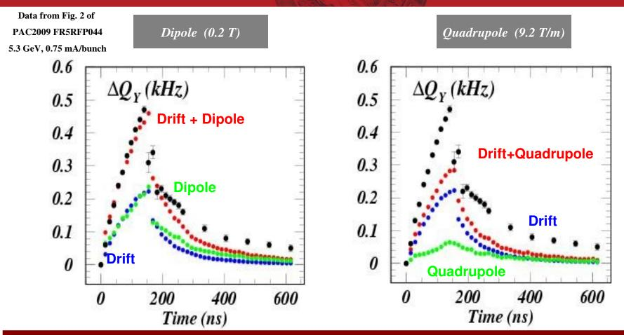
The assumption of dipole ring averages (61.5% occupancy and 1.16 photons/m/e) exaggerates the quadrupole contribution (8.5%, 0.78 photons/m/e) by more than a factor of 10.
