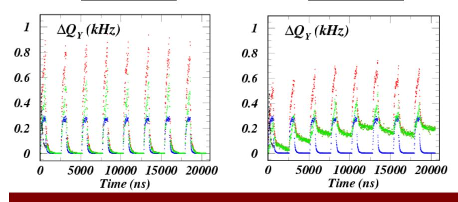
The cumulative effect slows after about six turns. Here only 45 of 183 bunches are filled.
