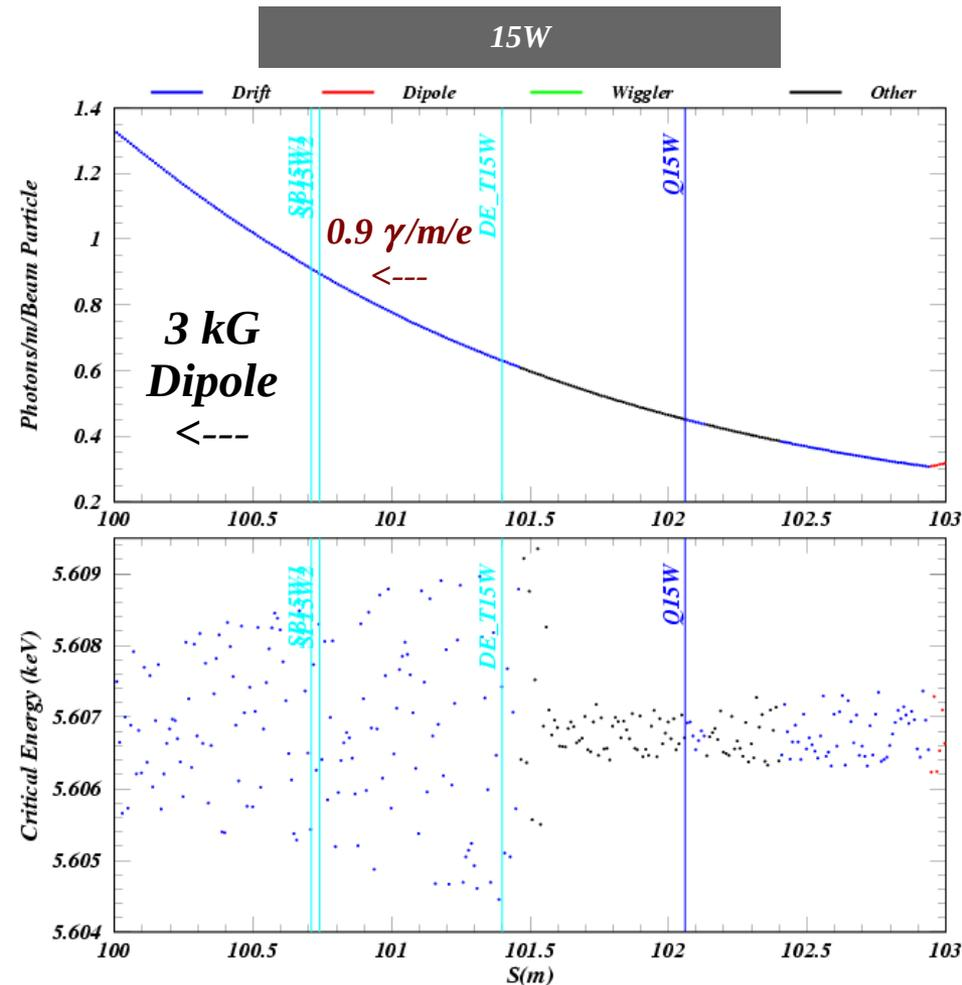
The 3 kG dipole is downstream (upstream) of the shielded button detector at 15E (15W) for the  $e^+$  beam.
