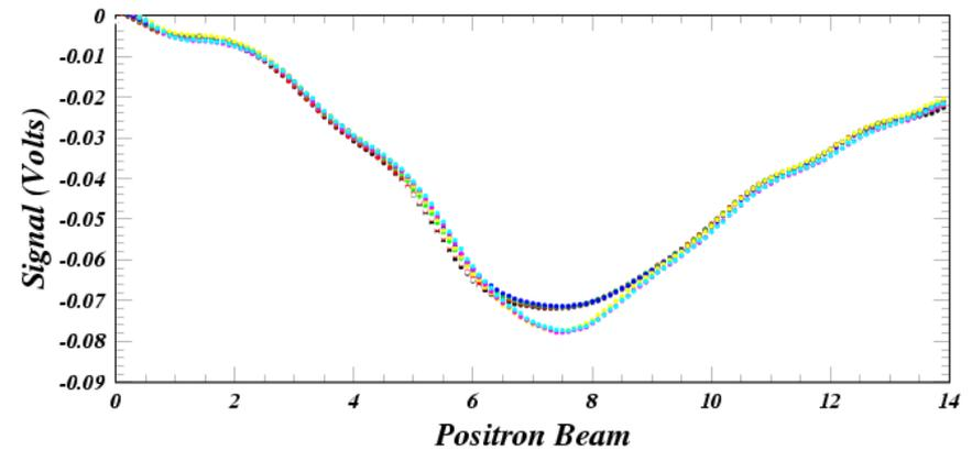
The parameterizations of the ECLLOUD photoelectron energy distributions have been adapted to reproduce the signal shapes. It was found that the risetime of the signal was dominated by primaries from the bottom of the vacuum chamber and that a higher-energy spectrum was required for  $e^-$  relative to  $e^+$  in order to overcome the beam kick.
