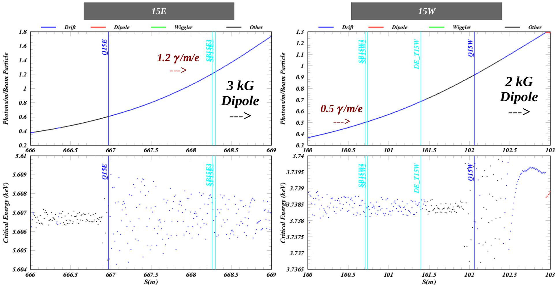
The 3 kG dipole is upstream (downstream) of the shielded button detector at 15E (15W) for the  $e^-$  beam.
