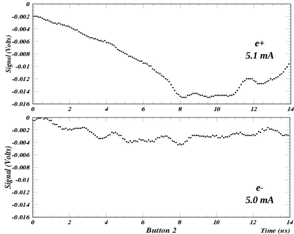
*Using a more appropriate scale to compare the e+ and e- signal magnitudes at 15W shows more clearly that the ratio  $0.035/0.15 = 0.23$  is consistent with the value 0.27 expected from the assumption that the reflectivity ratio is similar to what was found at 15E, and inconsistent with the value of 0.1 resulting from the assumption that the reflectivity is associated with the direction of the beam rather than the species.*
