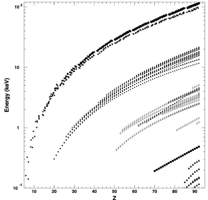
Fig. 4. Energy of fluorescence photons generated by Geant4 Atomic Relaxation as a function of the atomic number  $Z$ ; the symbols represent transitions originating from a vacancy in the K shell (stars), L shell (dots), M shell (diamonds), N shell (squares), and O shell (triangles); for better readability the plot shows K, L, and M transitions with probability  $> 10^{-3}$ , N transitions with probability  $> 5 \cdot 10^{-4}$  and O transitions with probability  $> 10^{-6}$ .
