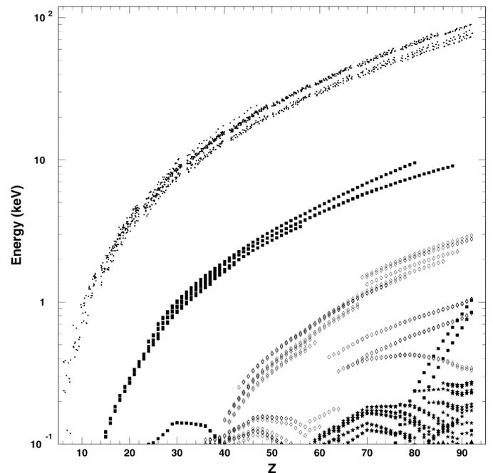
Fig. 5. Energy of electrons generated by Geant4 Atomic Relaxation as a function of the atomic number  $Z$ ; the symbols represent Auger and Coster-Kronig transitions originating from a vacancy in the K shell (dots), L shell (squares), M shell (diamonds), N shell (stars), and O shell (triangles); for better readability the plot shows K transitions with probability  $> 10^{-3}$  and L, M, N and O transitions with probability  $> 0.1$ .
