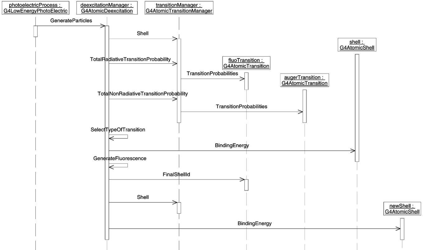
Fig. 3. The UML sequence diagram illustrates the most significant messages concerning the generation of atomic relaxation exchanged among objects of the Atomic Relaxation package.
