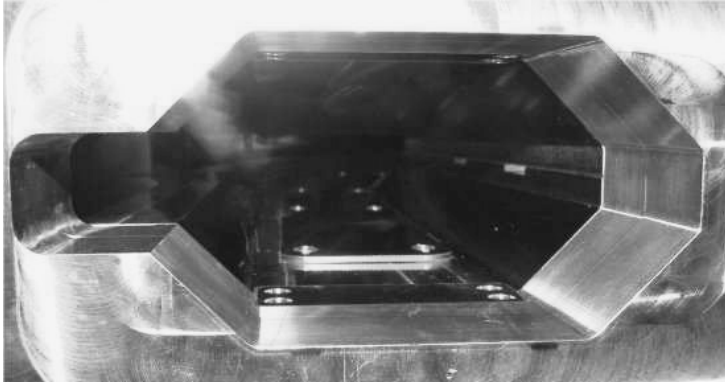
Figure 13. Left: clearing electrode in a DAΦNE dipole vacuum chamber; right: electron intensity grow rate (Figs. 5 and 14 in Ref [90], respectively).
