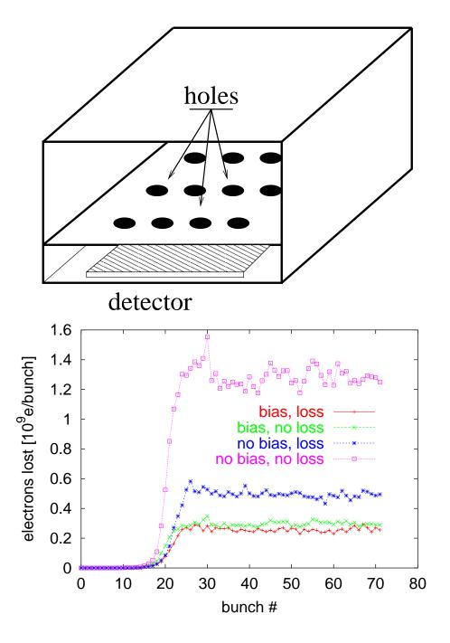
ullet Strip detector in dipole field,  $\delta_{max}=1.5$ , r=1
