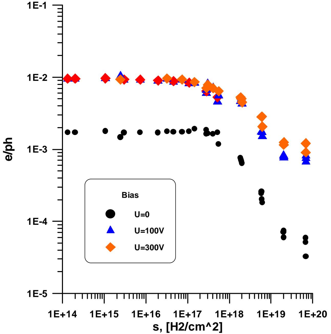
Figure 3. Photoemission from CO2 condensed at ~68K on the stainless steel substrate
