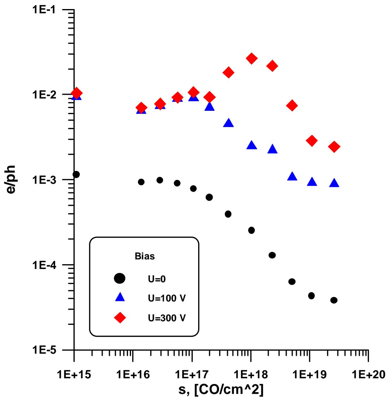
Figure 6. Photoemission from Ar condensed at 4.2K on the stainless steel substrate
