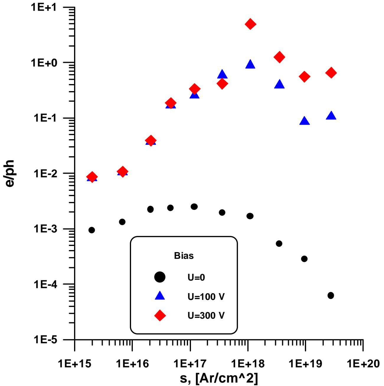
Figure 7. Photoemission from condensed gases on the stainless steel substrate
