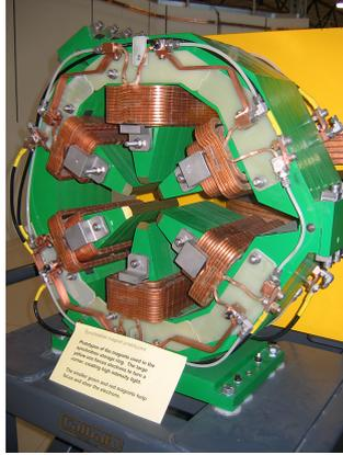
Figure 3: A sextupole magnet in Australian Synchrotron [1].
