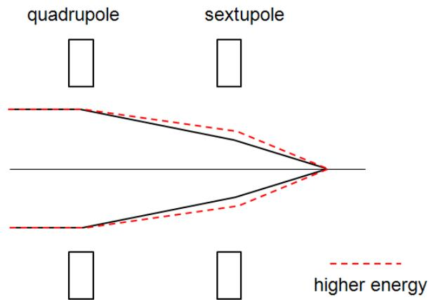
Figure 2: How a sextupole magnet works.
