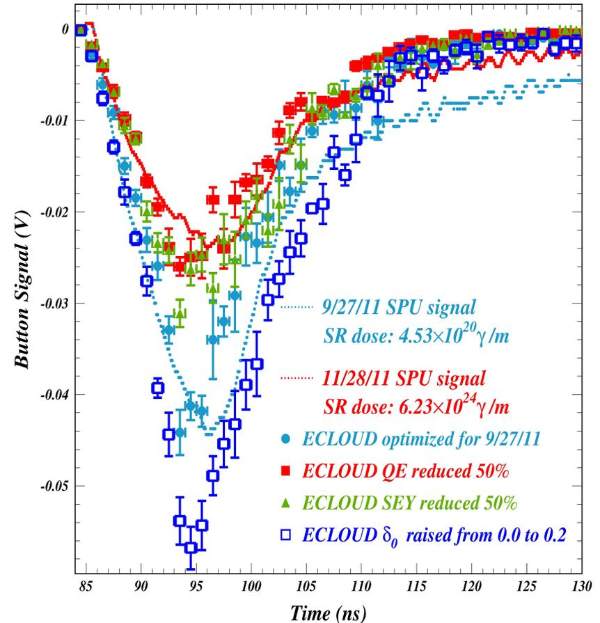
Conditioning effect for a previously unprocessed a-C coating affects the quantum efficiency, not the SEY, as for the late conditioning process.
