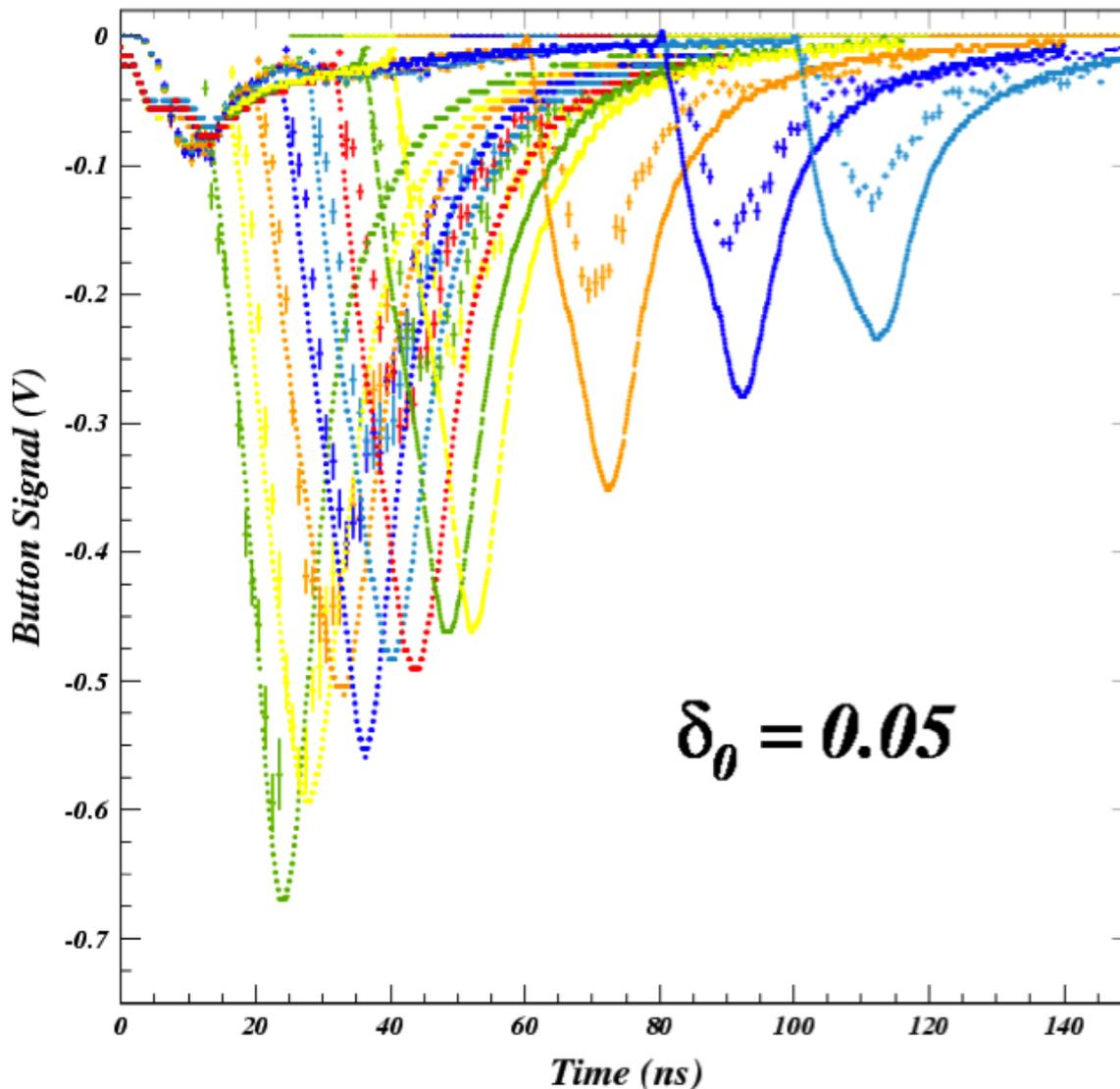
**Superposition of eleven two-bunch SPU signals with time delays between 12 and 100 ns, compared to the ECLLOUD model result**
