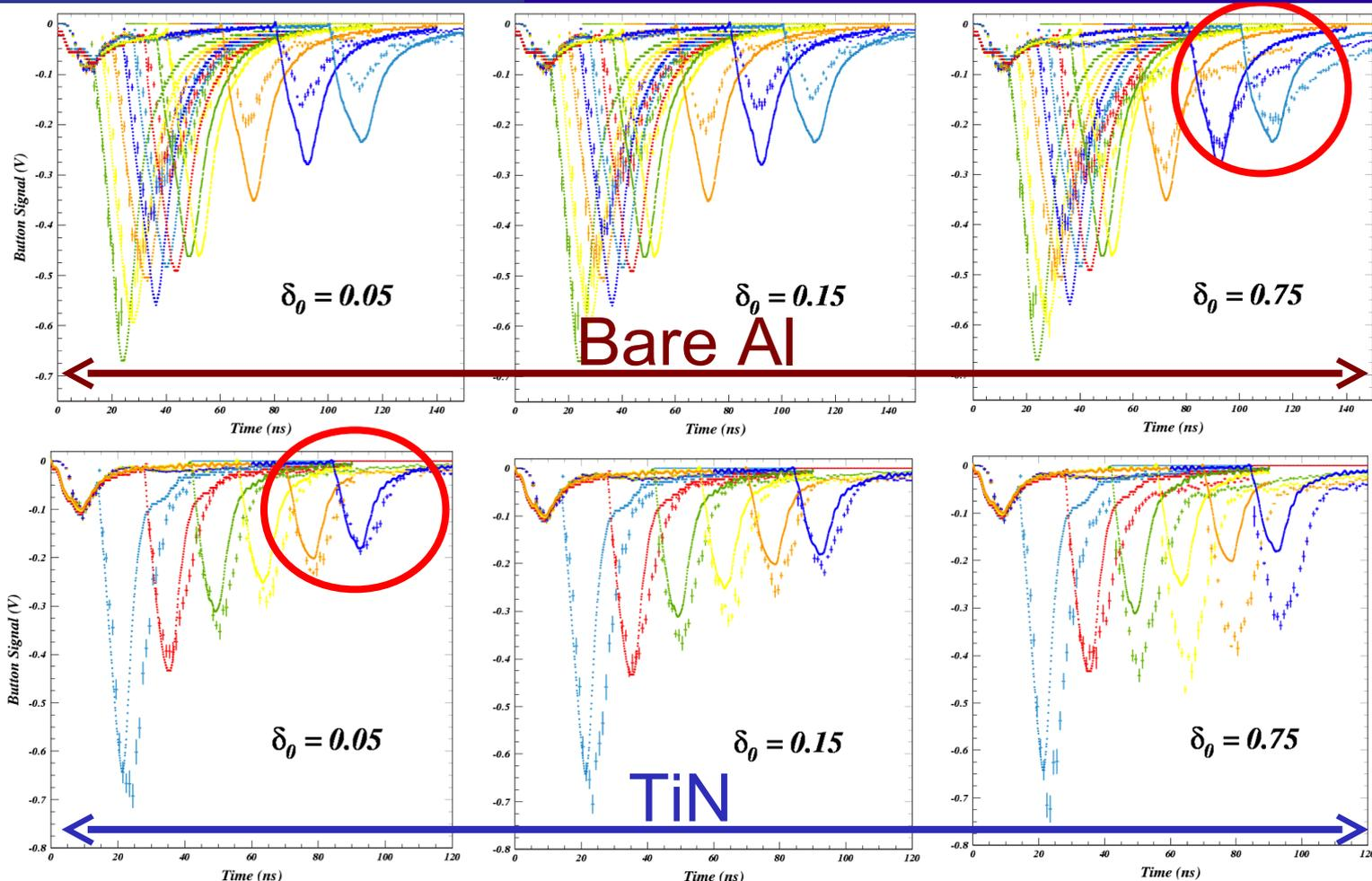
Witness bunch studies with delays up to 100 ns show clear sensitivity to the secondary elastic yield parameter, giving a value of about 0.75 for bare aluminum and about 0.05 for the TiN coating. The discriminating power is independent of the photoelectron model.
