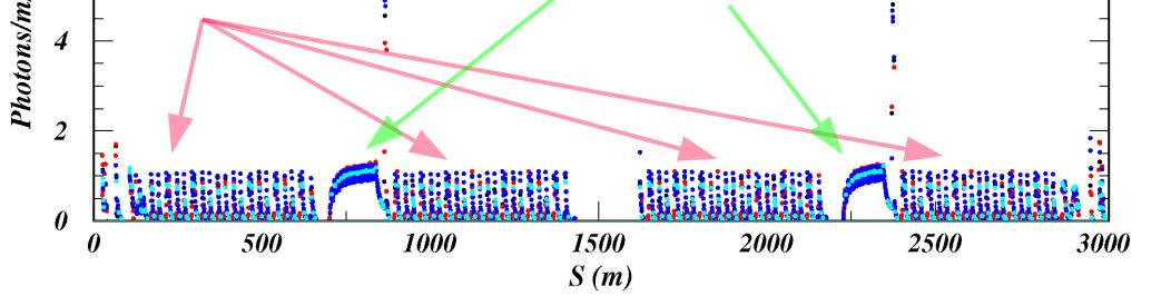
Synchrotron radiation photon absorption rates around the entire positron ring including the effects of reflection and scattering
