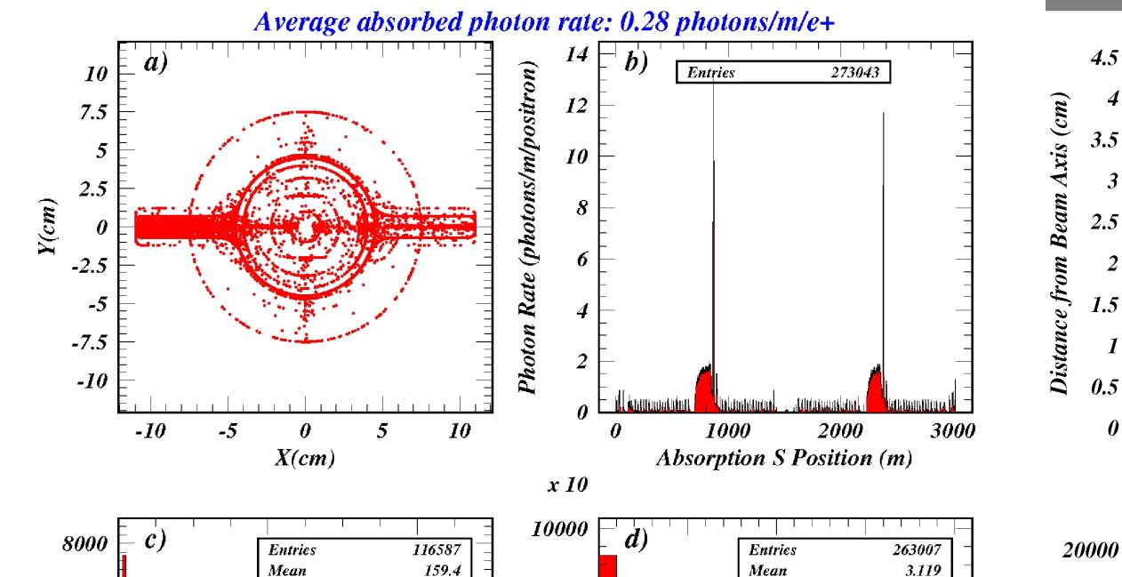
The figure below shows the characteristics of scattered and reflected photons absorbed within 10 m of the IP. The rate is particularly high in the region of the QC1RP magnet just upstream of the IP, higher than in the wiggler regions of the ring.
