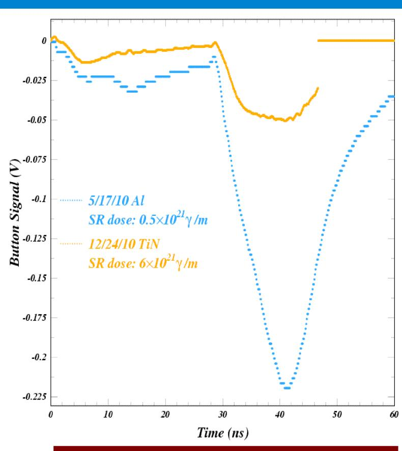
The quantum efficiency for reflected photons and the secondary yield are both much smaller for conditioned TiN than for uncoated aluminum.
