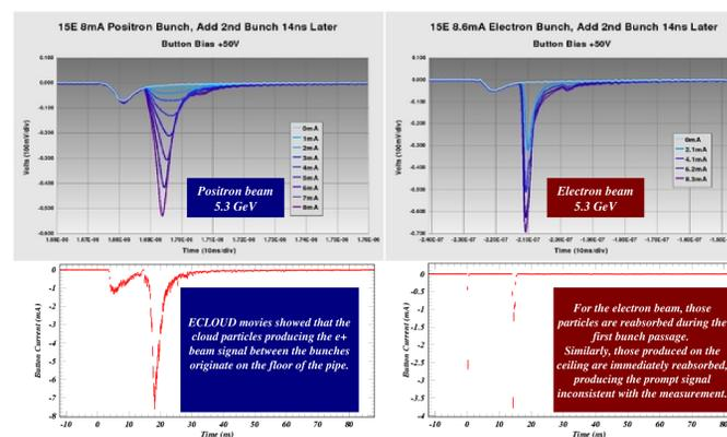
E-CLOUD fails to model the signal for an electron beam with high bunch current, because the production energies of the photoelectrons are too low to overcome the repulsion of the beam kick.
