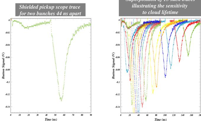
The single bunch signal arises from photoelectrons produced on the bottom of the vacuum chamber. Its shape is thus closely related to the photoelectron kinetic energy distribution modulo the beam kick.
