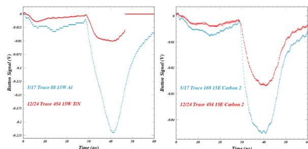
The second carbon-coated chamber shows conditioning effects between 5/17 and 12/24, primarily for the quantum efficiency.
