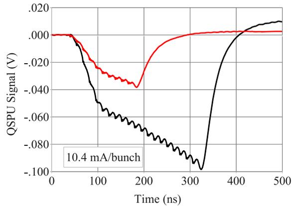
Figure 4: Quadrupole shielded electrode data from a 10-bunch train and a 20-bunch train of positrons at 10 mA/bunch ( $1.6 \times 10^{11}$  positrons/bunch).
