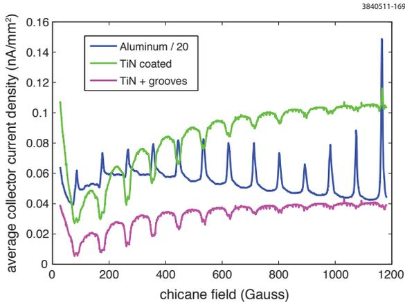
Figure 11: RFA signal as a function of dipole field:  $1 \times 451$  mA positrons, 5 GeV 4 ns spacing. Cyclotron resonances are observed every 89 G. Note that the Aluminum chamber signal is divided by 20.
