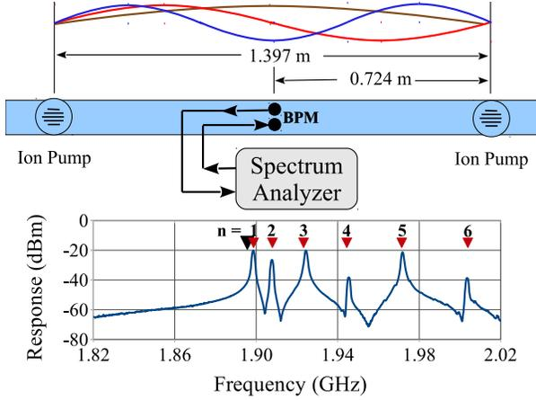
Figure 7: An example of resonant response of CESR beam-pipe. The triangles mark the resonant frequencies calculated for a shorted section of waveguide of length 1.385 m with a cutoff frequency of 1.8956 GHz.
