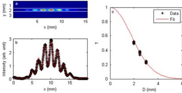
Figure 17: A typical interference pattern of SR using a  $D=2.0$  mm double slits. (b) The horizontal intensity profile integrated between two white lines in (a) and the best fit using Eq. (1). (c) The visibility measured using three different sets of double slits ( $D=2.0, 2.5,$  and  $3.0$  mm).
