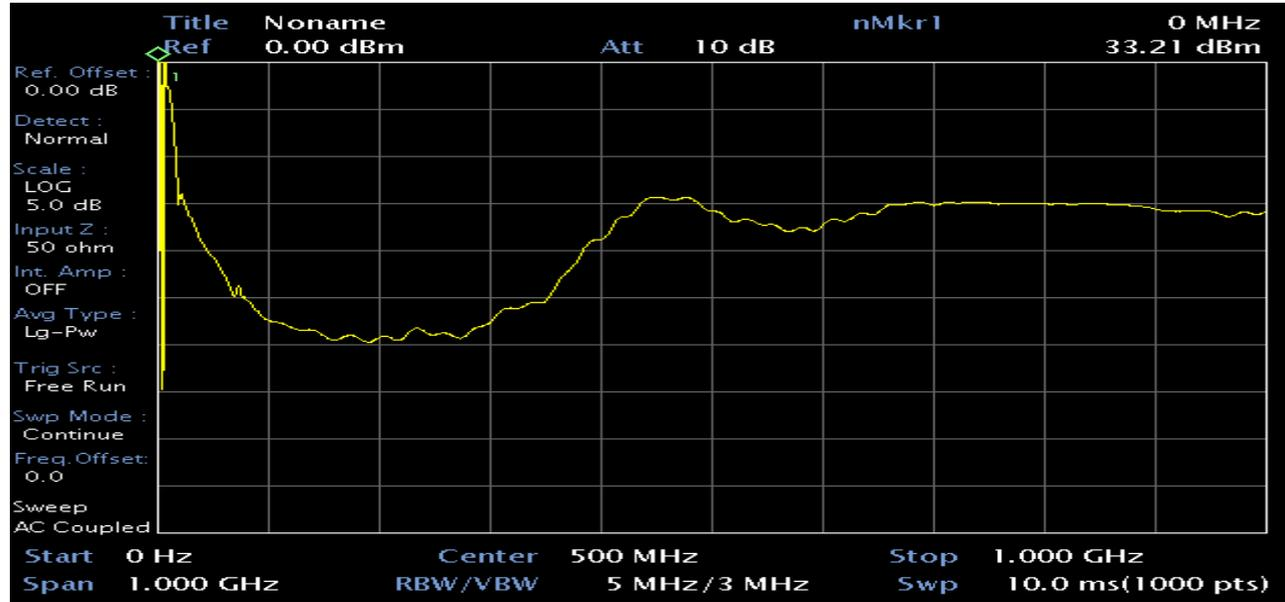
Simulated  $S_{21}$  of the stripline detector with 10 mm electrode (5 dB/div)
