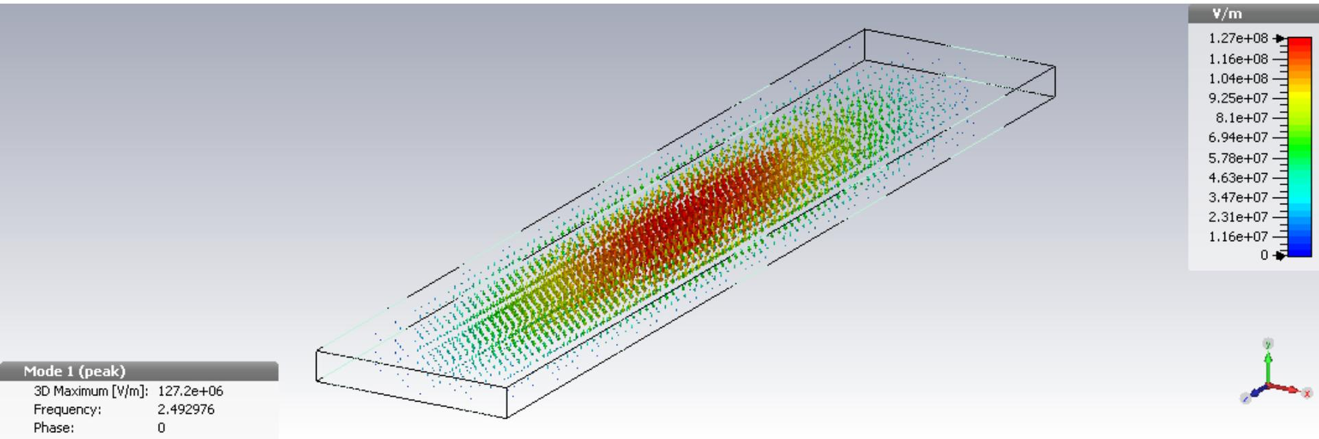
With the ceramic in empty space, the first resonant mode is at 2.5 GHz
