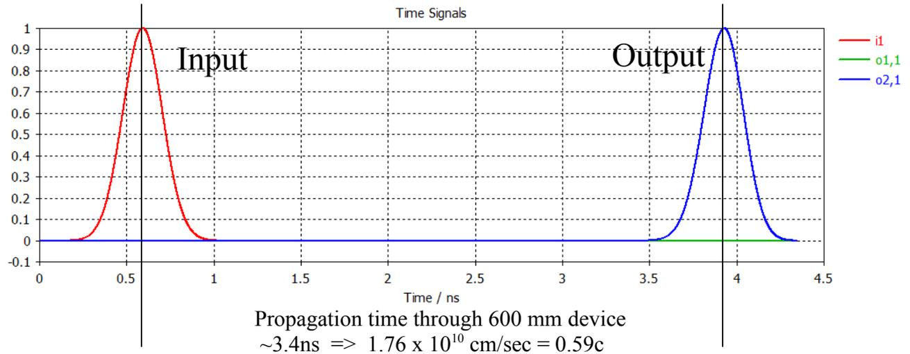
Stripline with tapers to 10 mm electrode on Kapton
