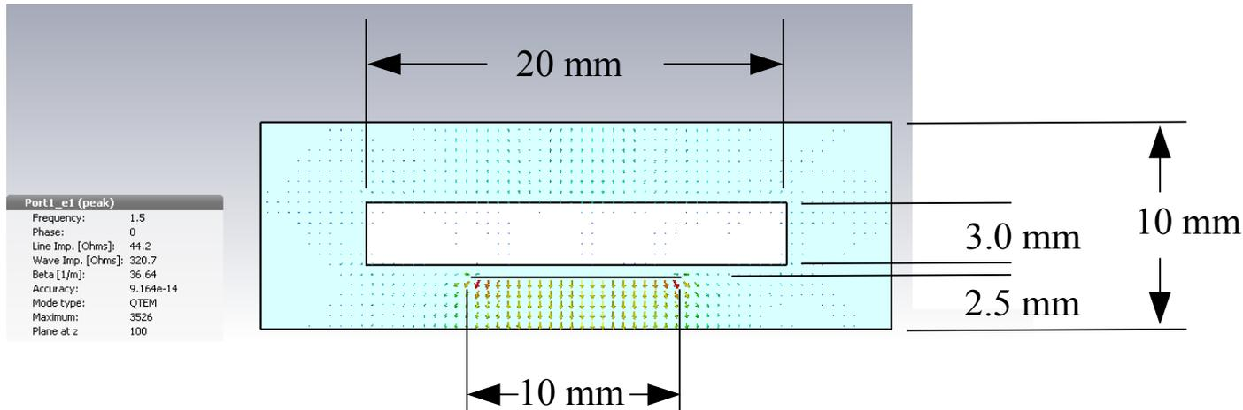
Stripline Simulations: Adding 3 mm thick ceramic results in 15 mm total height and a 3.5 mm collector gap for 50  $\Omega$ .
