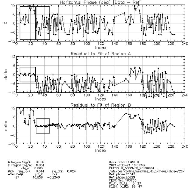
Figure 2: Results of a wave analysis applied to the difference in measured phase function for two sextupole strength settings which differ by  $\Delta k_2 l = 1.25 m^{-2}$ . The upper plot shows the difference in the phase function, the middle plot show the residuals of the fit to the upstream 23 BPMs and the bottom plot shows the residuals of the fit to the 19 downstream BPMs.
