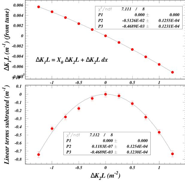
Figure 1: Quadrupole kick values calculated via  $\Delta k_1 l = \nu/\beta$  as a function of the change in sextupole strength  $\Delta k_2 l$ . The initial offset  $X_0$  is determined to be  $5.126 \pm 0.013$  mm. The quadratic term shows the dependence of the orbit change in the sextupole on the change in its strength. The lower plot shows the dependence with the linear term subtracted, observed to be purely parabolic to good accuracy.
