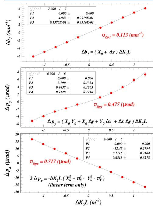
Record phase and orbit measurements for eleven sextupole settings. Reference the ten sets of measurements with nonzero  $K_2$  settings to the  $K_2=0$  orbit and phase measurements. Fit for the linear terms in  $\Delta b_1(\Delta k_2l)$ ,  $\Delta x'(\Delta k_2l)$ ,  $\Delta y'(\Delta k_2l)$ .
