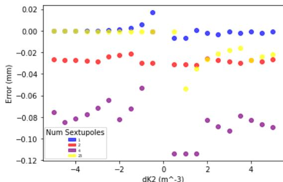
Figure 5. Error in beam size calculation as a function of sextupole strength change, for multiple sextupoles in a ring. Constant  $X_{mis} = .9 \text{ mm}$  and  $\sigma_{in} = 2.1 \text{ mm}$ .
