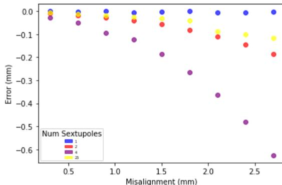
Figure 4. Error in beam size calculation as a function of misalignment, for multiple sextupoles in a ring. Constant  $\Delta K_2 = 3 \text{ m}^{-3}$  and  $\sigma_{in} = 2.1 \text{ mm}$ .
