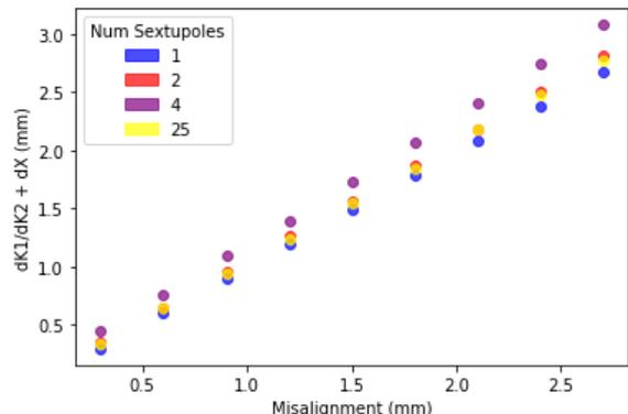
Figure 7.  $X_0$  evaluated using tune data vs. initial misalignment of sextupole, for constants values of inputted beam size  $\sigma_{in} = 2.1 \text{ mm}$  and sextupole strength change  $\Delta K_2 = 3 \text{ m}^{-3}$ .
