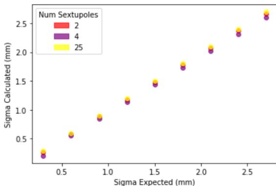
Figure 3. Calculated vs. Expected beam size using tune data, for a constant value of  $X_{mis} = 1.2 \text{ mm}$  and  $\Delta K_2 = 3 \text{ m}^{-3}$ . Different colors represent data for lattices with different numbers of sextupoles.
