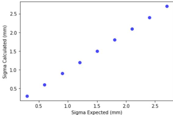
Figure 2. Calculated vs. Expected beam size using tune data, for a constant value of  $X_{mis} = 1.2 \text{ mm}$  and  $\Delta K_2 = 3 \text{ m}^{-3}$ .
